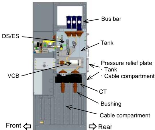
Fig. 3 Configuration of HS-X type C-GIS
