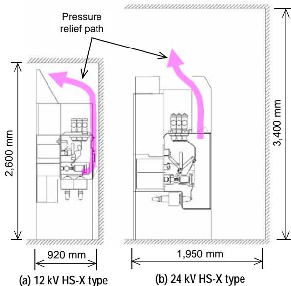
Fig. 5 Internal arc pressure relief path and electric room outline
