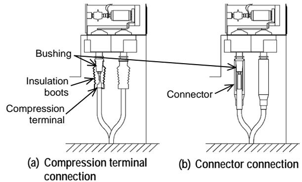
Fig. 6 Cable connection
