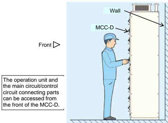
**Fig. 2 Front-access operation and maintenance**
