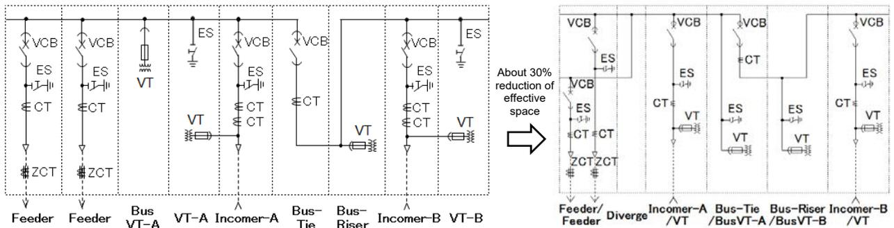
Fig. 3 Model arrangement comparison (conventional product on the left and MS-E on the right)
