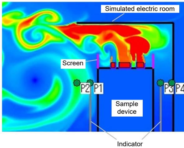
Fig. 7 Example results of hot air fluid analysis
