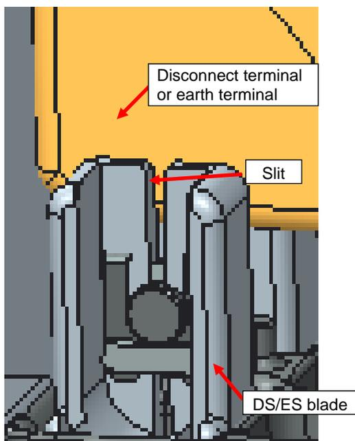
Fig. 3 Structure of DS/ES contact part
