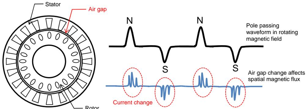
Fig. 8 Detection principle
