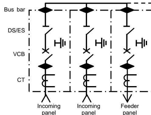
Fig. 2 C-GIS arrangement for C/S in closed-ring system
