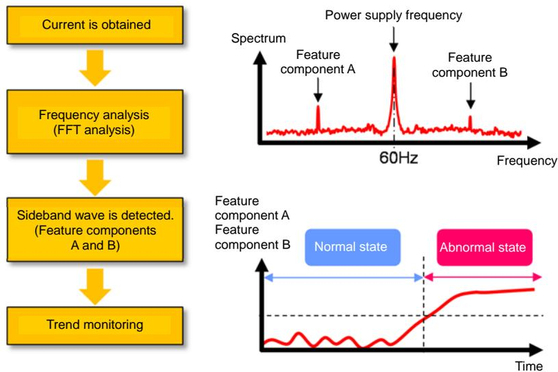
Fig. 9 Mechanical system abnormality detection technique
