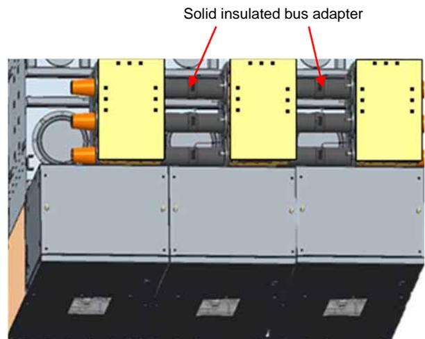
Fig. 7 Top view after panel arrangement
