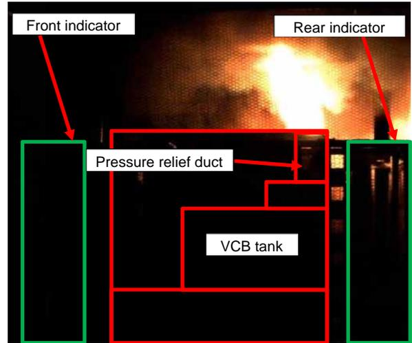
Fig. 5 Scene from type testing during arc accident inside VCB tank
