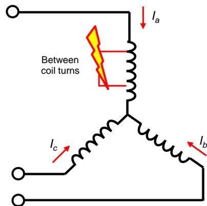
Fig. 10 Principle of layer short
