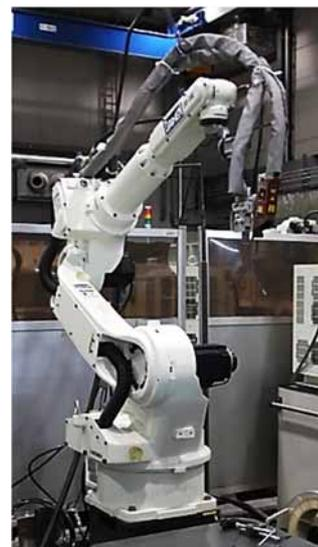
Fig. 7 Robot welder
