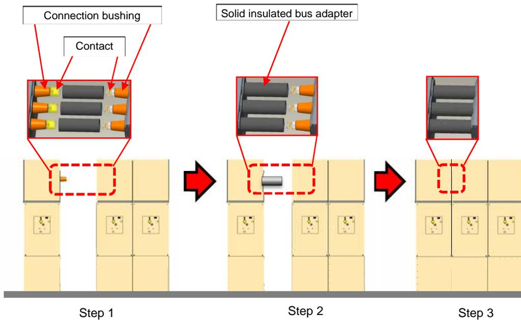
Fig. 6 Arrangement of solid insulated bus
