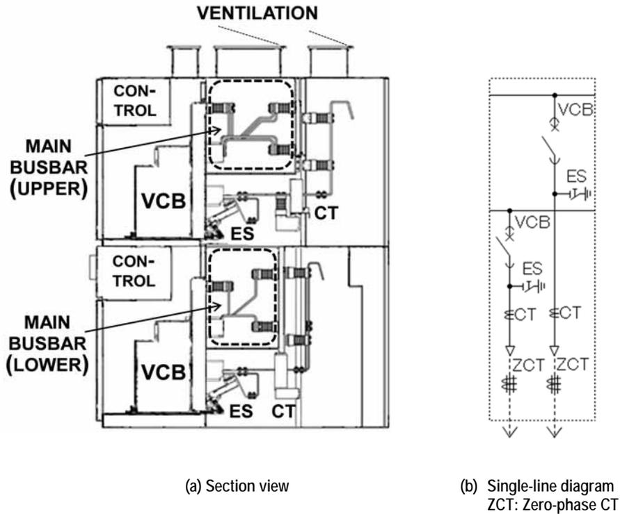
Fig. 2 Section view and single-line diagram of MS-E feeder panel
