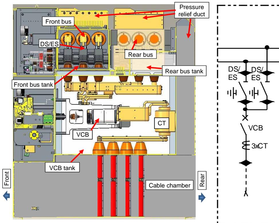
Fig. 1 Cross-sectional view and skeleton diagram of C-GIS Type “HS-X”
