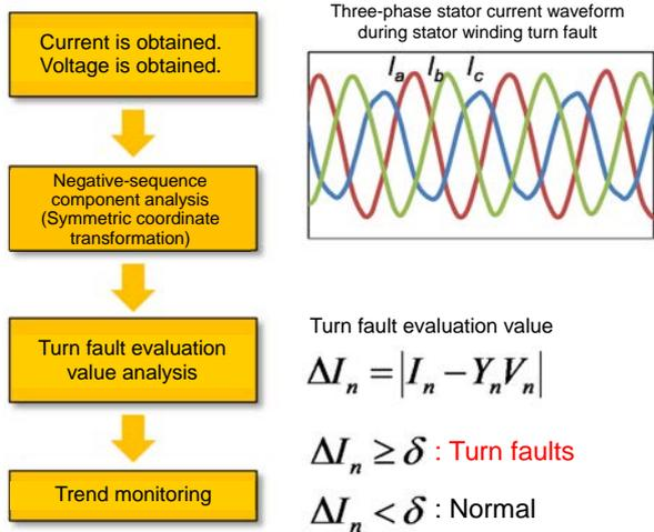
Fig. 11 Stator winding turn fault detection technique
