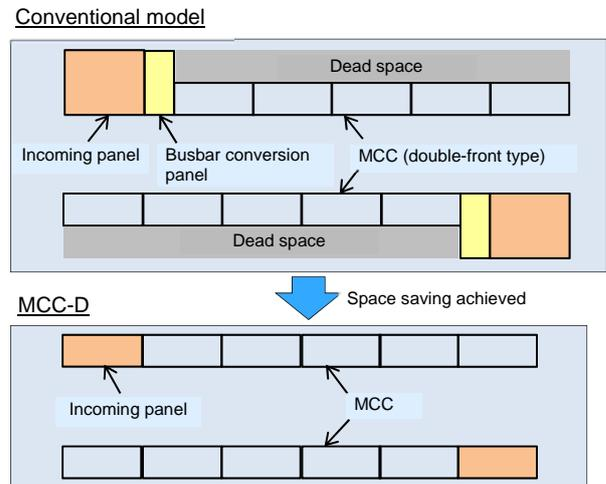
**Fig. 5 MCC layout in a container-type substation (top view)**
