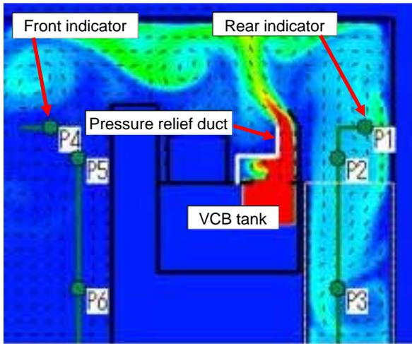
Fig. 4 Results of hot air fluid analysis during an arc accident inside a VCB tank
