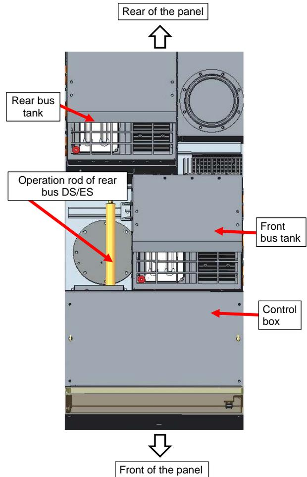
Fig. 2 Top view of double bus configuration of C-GIS Type "HS-X"
