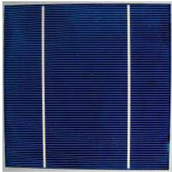
Polycrystalline silicon PV cell
