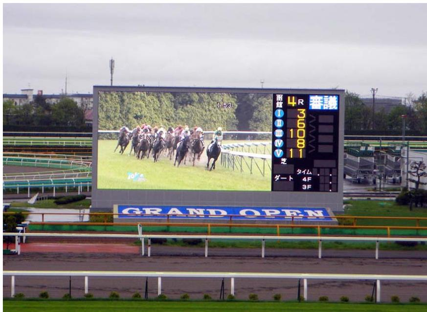
The main display features high-luminance light-emitting diodes (LEDs) aligned in a 10 mm dot pitch (see “Specifications” below). The split-screen display can simultaneously showcase two screens of content, such as live footage of a race or the paddock on one screen and race odds and other data on the other.
