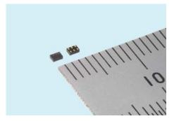
The MGF7301 is the first amplifier of its kind to include external matching elements such as capacitors and inductances. Its 0.75dB low-noise level is achieved with miniaturized transistors, and improves signal reception. The amplifier includes a stand-by mode to save power consumption when GPS is not used.
