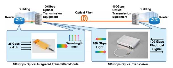
Mitsubishi Electric's optical transmission technologies enable 100 Gbps optical transmission per wavelength thanks to its newly developed integrated optical transmitter module and optical transceiver, which are installed to 100 Gbps optical transmission equipment. Transmission capacity per power consumption is 40% more efficient compared to existing devices due to effective integration of the optical module and other key components.
