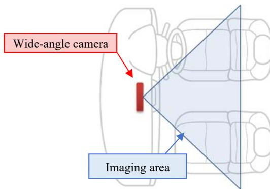
Flexible installation of camera position
