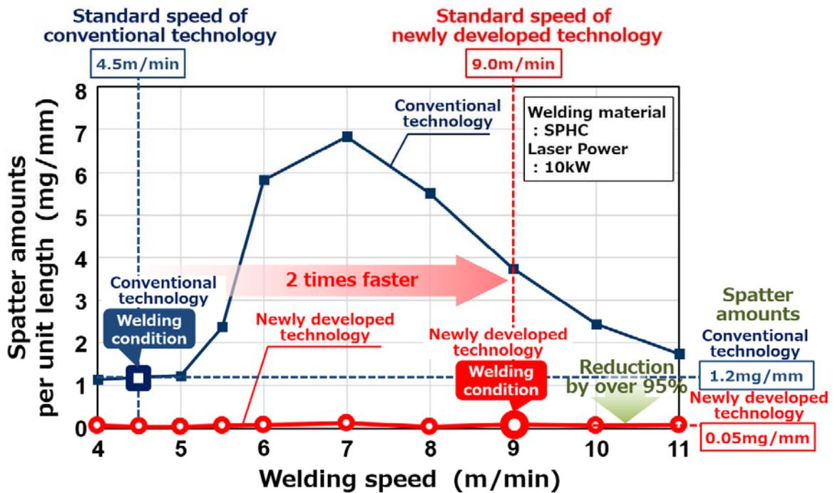
Fig. 3. Comparison of spatter amounts
