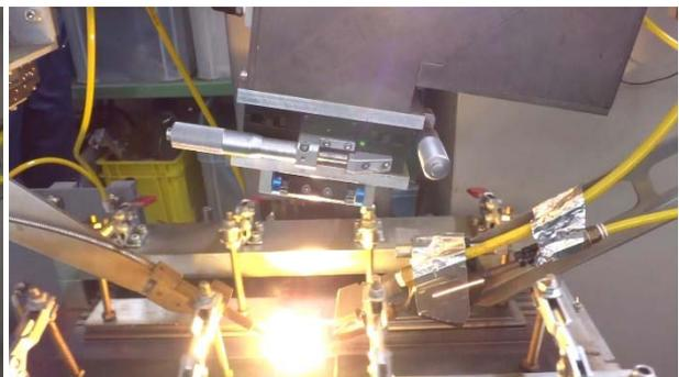
Fig. 1. Visual comparison of spatter during fiber-laser welding
