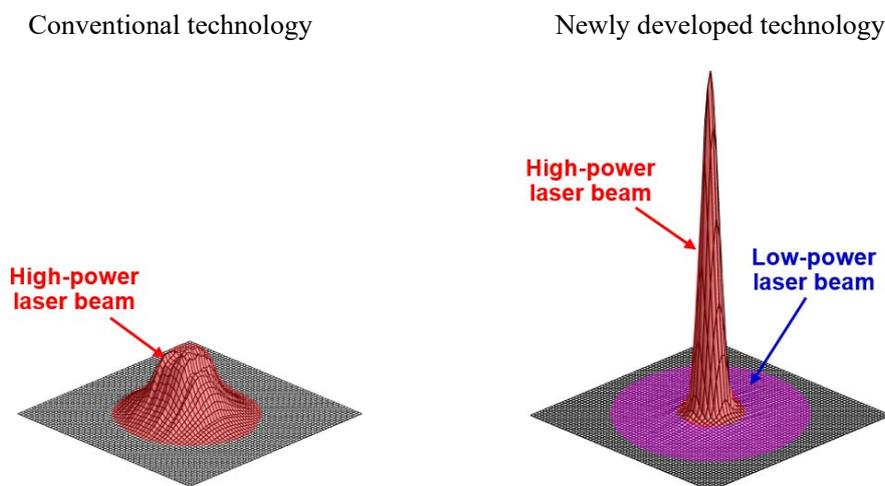
Fig. 2. Comparison of light-intensity distribution of focused laser beams
