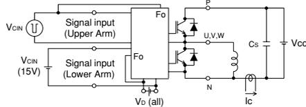
Fig. 3 Switching time and SC test circuit
