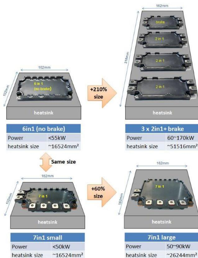
Figure 4: Heatsink size and inverter power comparison
