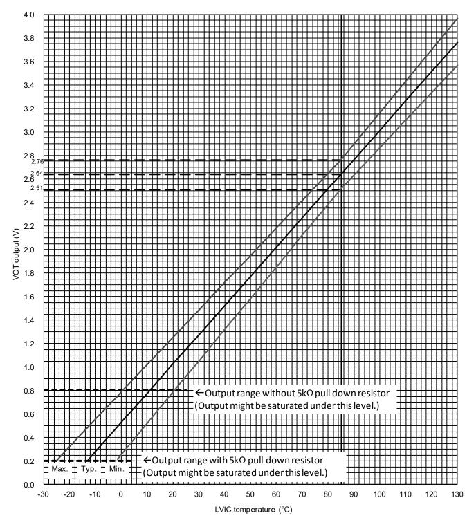
Fig.2-2-12 Vot output vs. LVIC temperature
