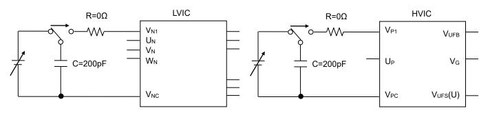
Fig.3-3-3 LVIC terminal Surge Test circuit
