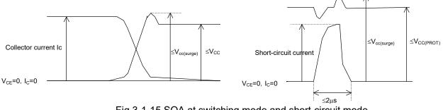
Fig.3-1-15 SOA at switching mode and short-circuit mode
