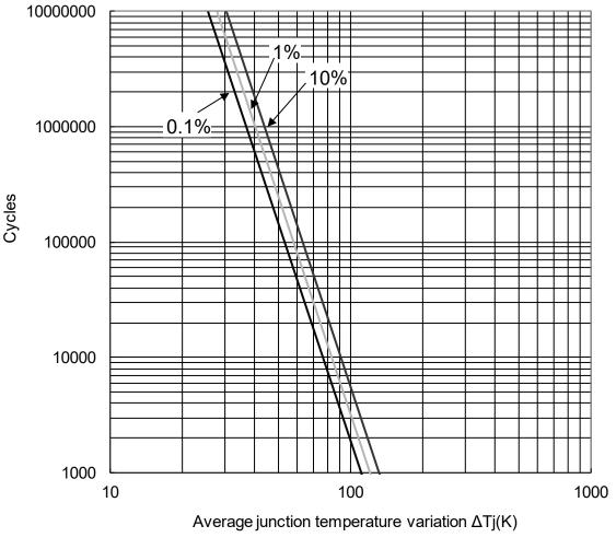
Fig.3-1-18 Power cycle curve
