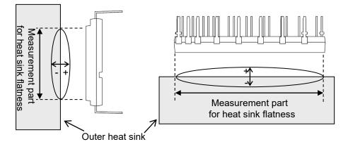
Fig.2-4-2 Measurement point of heat sink flatness(PSSxxS71F6)
