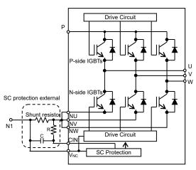
Fig.2-2-1 SC protecting circuit
