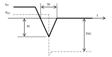
Fig.3-2-1 Ideal FWDi recovery characteristics curve
