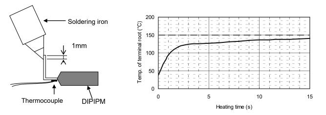
Fig.2-4-3 Heating and measuring point Fig.2-4-4 Temperature alteration of the terminal root (Example)
