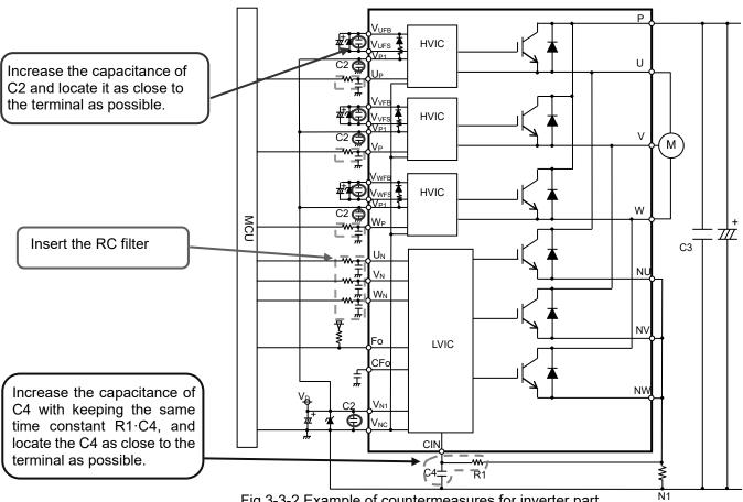
Fig.3-3-2 Example of countermeasures for inverter part
