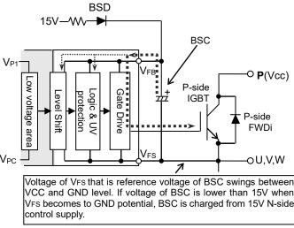
Fig.4-1-2 Bootstrap Circuit Diagram
