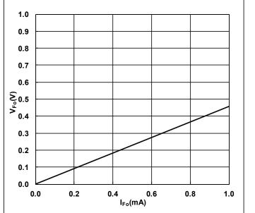
Fig.3-1-8 Fo terminal typical V-I characteristics ( $V_D$ =15V,  $T_j$ =25°C)
