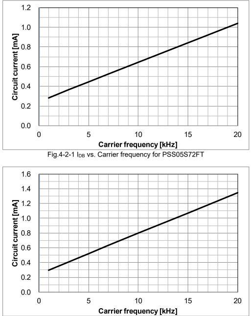
Fig.4-2-2 IDB vs. Carrier frequency for PSS10S72FT
