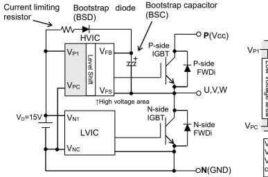
Fig.4-1-1 Bootstrap Circuit Diagram
