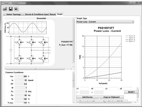
Fig.3-2-3 Loss simulator screen image
