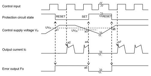
Fig.2-2-4 Timing chart of N-side UV protection
