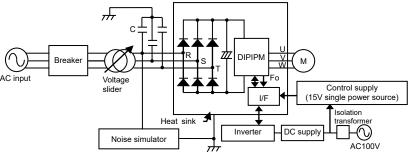
Fig.3-3-1 Noise withstand capability evaluation circuit
