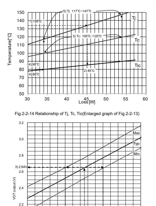
Fig.2-2-15  $V_{OT}$  output vs. LVIC temperature (Enlarged graph of Fig.2-2-12)
