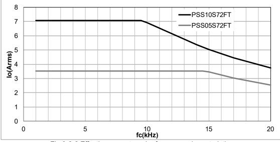
Fig.3-2-2 Effective current-carrier frequency characteristics
