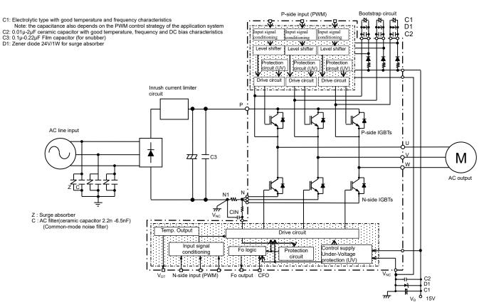
Fig.3-1-1 System block diagram (Example)
