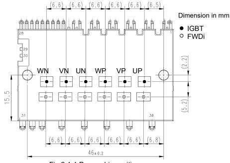
Fig.2-1-1 Power chip position
