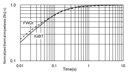
Fig.2-1-3 Typical transient thermal impedance (PSSxxS72FT)
