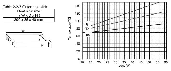
Fig.2-2-13 Example of relationship of Tj, Tc, Tic (One IGBT chip turns on. DC current Ta=25°C)
