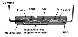
Fig.1-1-2 Internal cross-section structure
