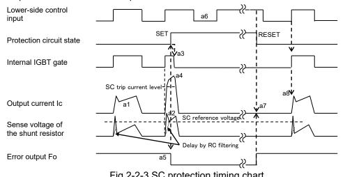
Fig.2-2-3 SC protection timing chart
