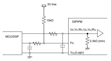
Fig.3-1-6 Control input connection
