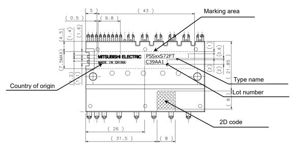
Fig.2-3-2 Laser marking view PSSxxS72FT (Dimension in mm)
