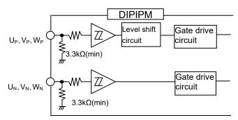
Fig.3-1-5 Internal structure of control input terminals
