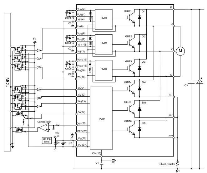
Fig.3-1-3 Interface circuit example with opto-coupler
