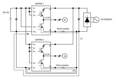
Fig.3-1-14 Parallel operation
