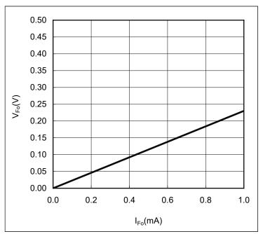
Fig.3-7 Fo terminal typical V-I characteristics ( $V_D$ =15V,  $T_i$ =25°C)
