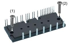
Fig.2-18 Recommended screw fastening order
