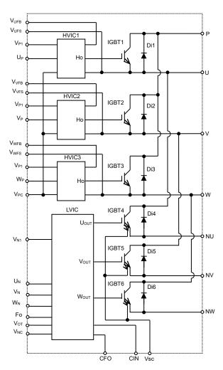
Fig.1-3 Internal circuit schematic
