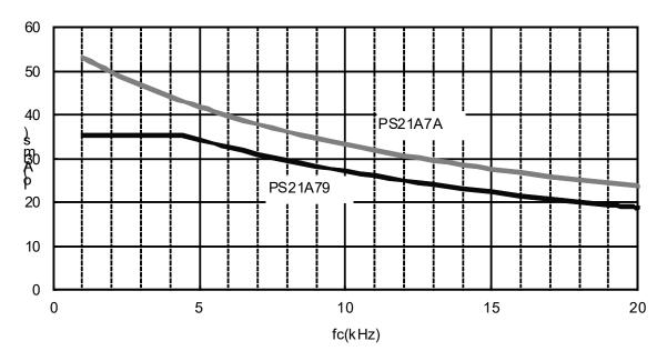
Fig.3-17 Effective current-carrier frequency characteristic
