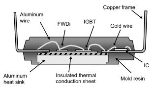
Fig.1-2 Internal cross-section structure
