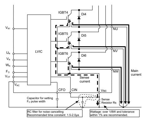
\*) This wattage of sense resistor is described as a guide, so it is recommended to evaluate on your real system well.
