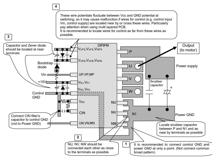
Fig.3-10 Precaution for wiring on PCB
