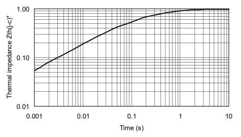
Fig.2-1 Typical transient thermal impedance
