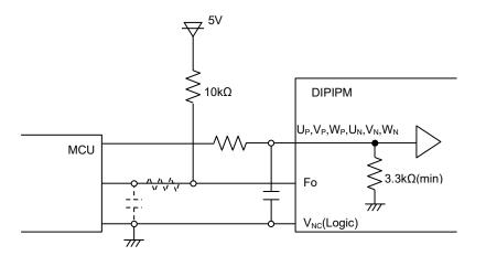
Fig.3-5 Control input connection
