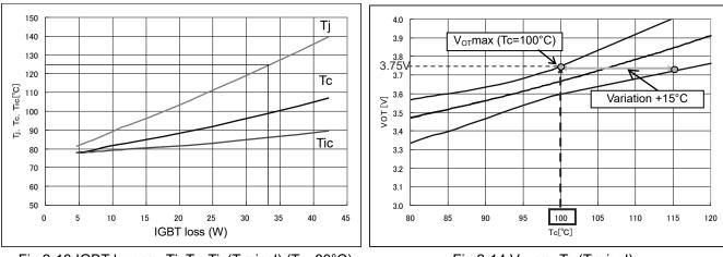
Fig.2-13 IGBT loss vs. Tj, Tc, Tic(Typical) (Ta=80°C)
