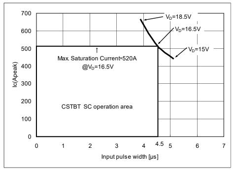
Fig.3-14 PS21A79 typical SCSOA curve
