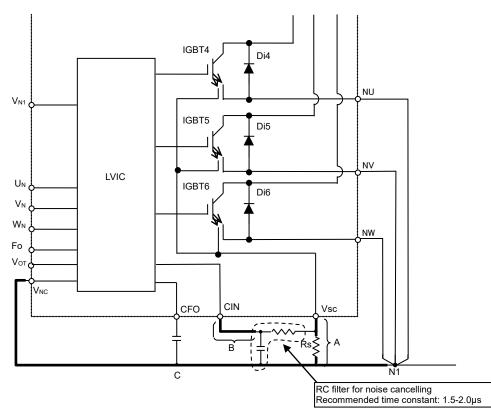
Fig.3-9 External protection circuit
