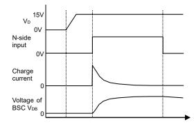
Fig.4-6 Example of waveform by one charging pulse
