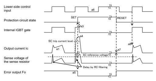
Fig.2-6 SC protection timing chart
