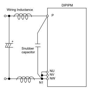
Fig.3-8 Recommended snubber circuit position
