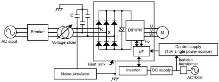
Fig.3-19 Noise withstand capability evaluation circuit
