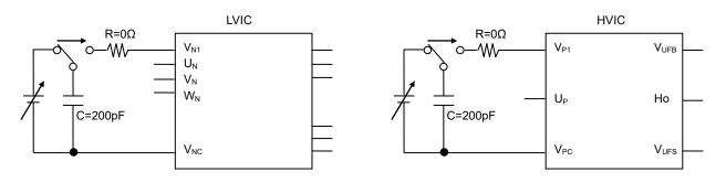
Fig.3-21 V<sub>N1</sub> terminal Surge Test circuit(V<sub>N1</sub> terminal)
