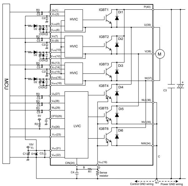
Fig.3-2 Interface circuit example (Direct coupling)
