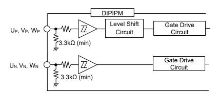
Fig.3-4 Internal structure of control input terminals
