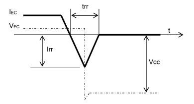
Fig.3-16 Ideal FWDi recovery characteristics curve
