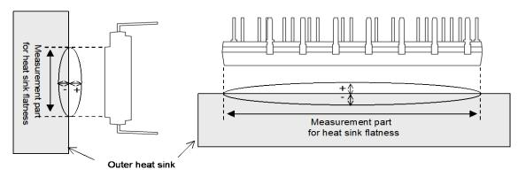
Fig.2-19 Measurement point of heat sink flatness
