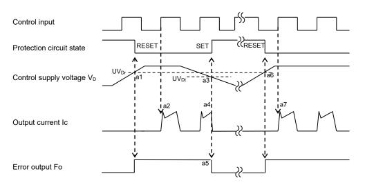
Fig.2-8 Timing chart of N-side UV protection
