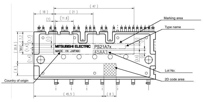
Fig.2-17 Laser marking view
