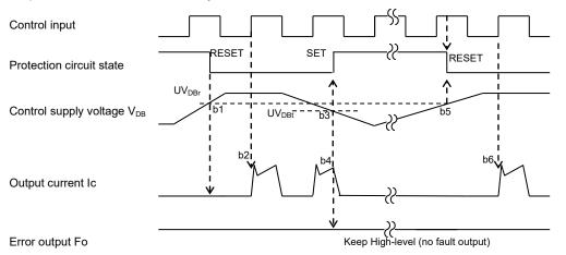
Fig.2-9 Timing Chart of P-side UV protection
