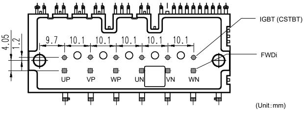
Fig.2-16 Power chip position
