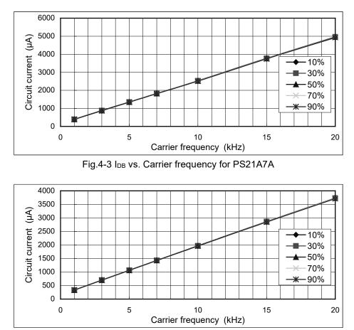
Fig.4-4 IDB vs. Carrier frequency for PS21A79
