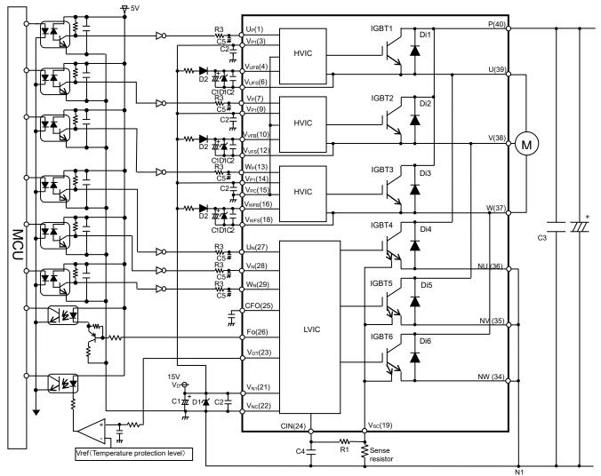
Fig.3-3 Interface circuit example with opto-coupler
