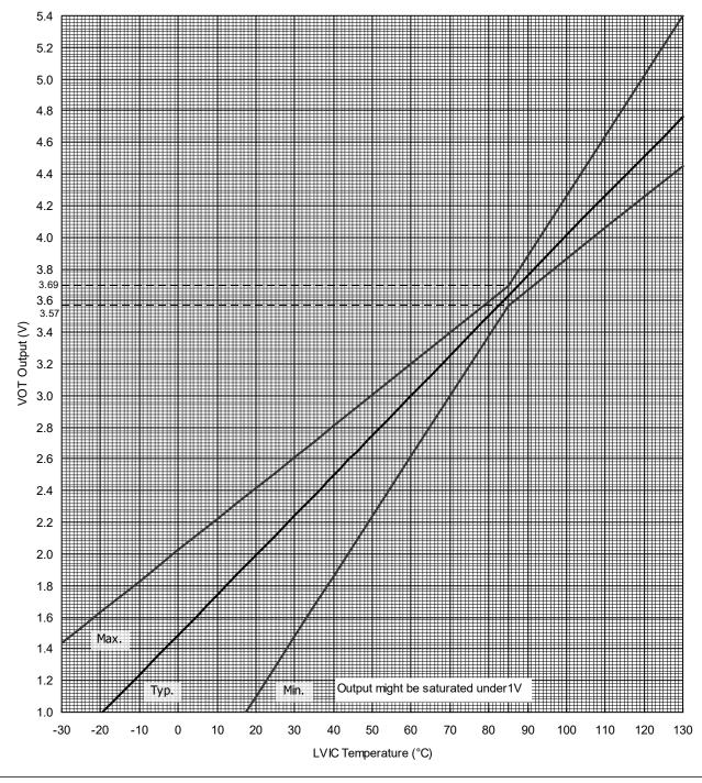
Fig.2-11 Vot output vs. LVIC temperature
