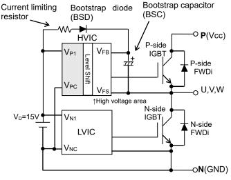
Fig.4-1 Bootstrap Circuit Diagram
