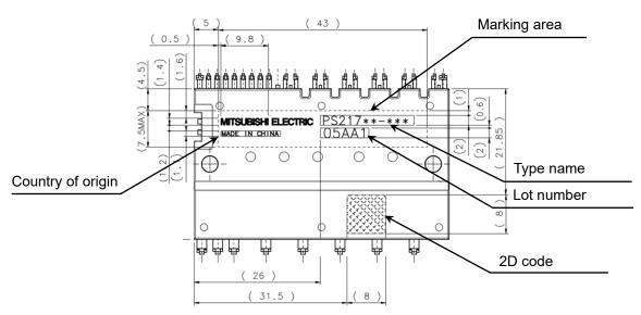
Fig.2-3-4 Laser marking view PSSxxS71F6 (Dimension in mm)
