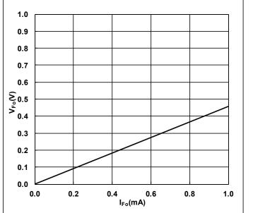
Fig.3-1-8 Fo terminal typical V-I characteristics ( $V_D$ =15V,  $T_j$ =25°C)
