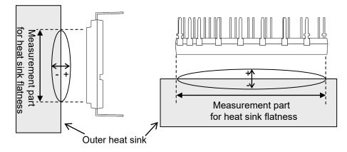
Fig.2-4-3 Measurement point of heat sink flatness (PSSxxS71F6)
