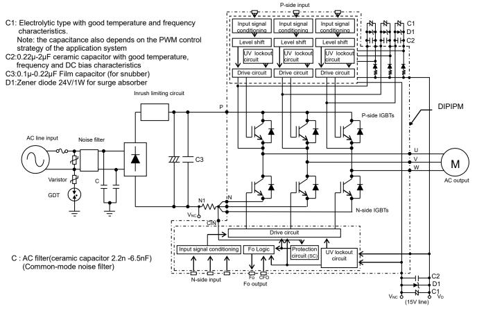
Fig.3-1-1 System block diagram (Example)
