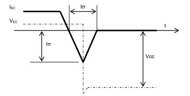
Fig.3-2-1 Ideal FWDi recovery characteristics curve
