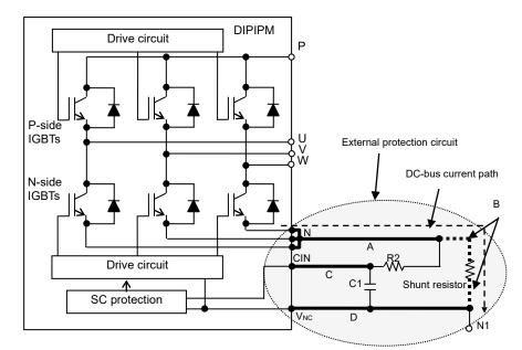
Influence of pattern wiring around the shunt resistor is shown below.
