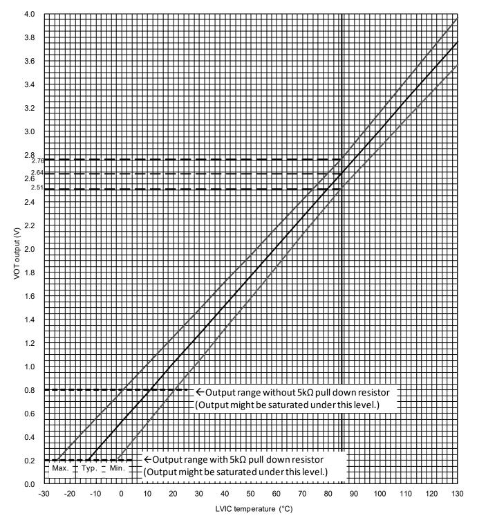
Fig.2-2-12 Vot output vs. LVIC temperature (PSSxxS71F6)
