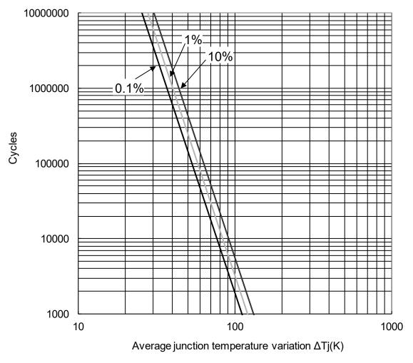
Fig.3-1-23 Power cycle curve
