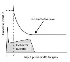
Fig.2-2-2 Filter time constant setting
