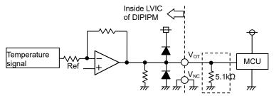
Fig.2-2-9  $V_{\text{OT}}$  output circuit in the case of detecting low temperature
