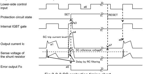
Fig.2-2-3 SC protection timing chart
