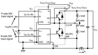
Fig.2-1-6 Evaluation circuit (inductive load) Short A for N-side IGBT, and short B for P-side IGBT evaluation
