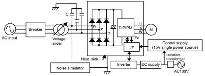
Fig.3-3-1 Noise withstand capability evaluation circuit
