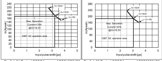
Fig.3-1-21 Typical SCSOA curve of PSS15S51F6 Fig.3-1-22 Typical SCSOA curve of PSS20S51F6
