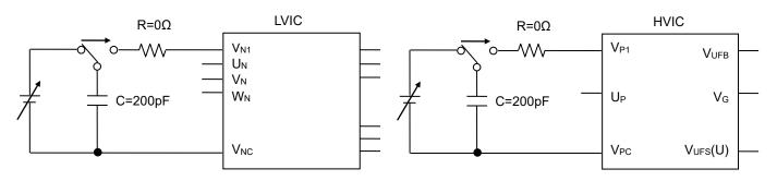
Fig.3-3-3 LVIC terminal Surge Test circuit
