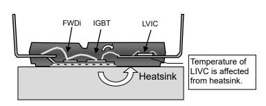
Fig.2-2-7 Thermal conducting from power chips
