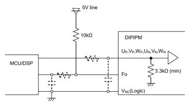
Fig.3-1-6 Control input connection
