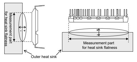
Fig.2-4-4 Measurement point of heat sink flatness (PSSxxS51F6)
