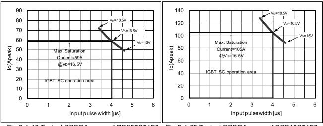
Fig.3-1-19 Typical SCSOA curve of PSS05S51F6 Fig.3-1-20 Typical SCSOA curve of PSS10S51F6
