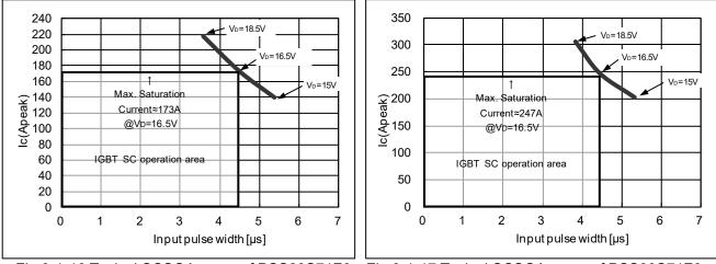
Fig.3-1-16 Typical SCSOA curve of PSS20S71F6 Fig.3-1-17 Typical SCSOA curve of PSS30S71F6
