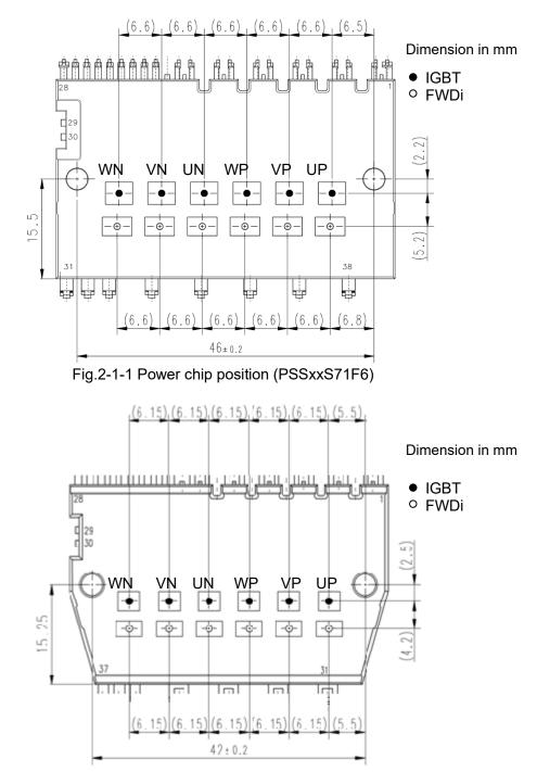
Fig.2-1-2 Power chip position (PSSxxS51F6)
