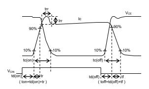
Fig.2-1-5 Switching time definition
