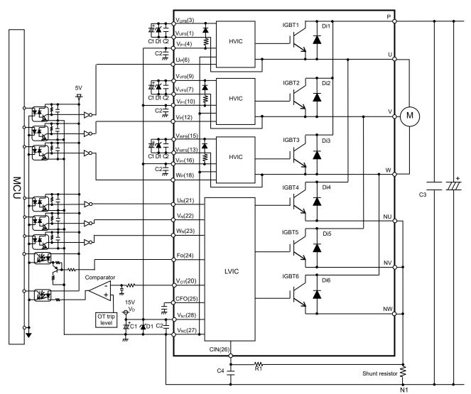
Fig.3-1-3 Interface circuit example with opto-coupler
