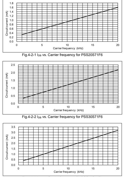
Fig.4-2-3 IDB vs. Carrier frequency for PSS50S71F6
