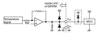
Fig.2-2-10 V<sub>OT</sub> output circuit in the case of using with low voltage controller
