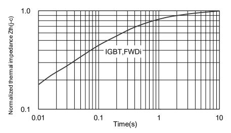
Fig.2-1-4 Typical transient thermal impedance (PSSxxS51F6)
