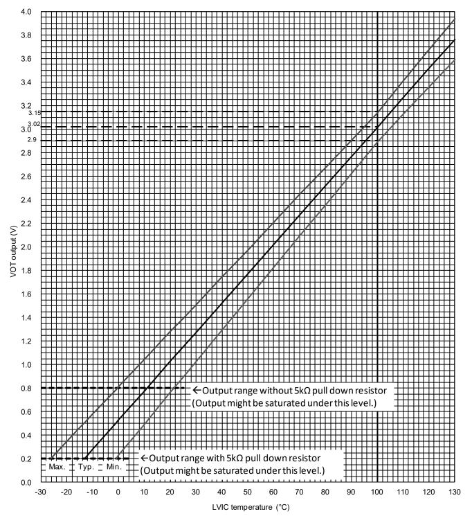
Fig.2-2-13 Vot output vs. LVIC temperature (PSSxxS51F6)
