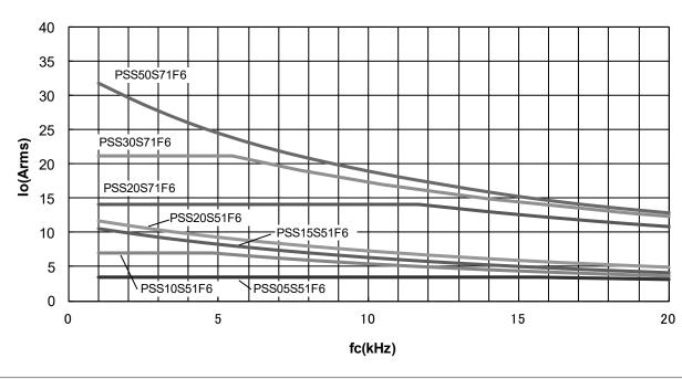
Fig.3-2-2 Effective current-carrier frequency characteristics
