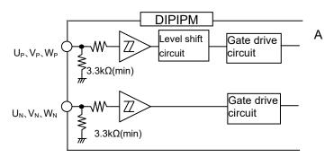
Fig.3-1-5 Internal structure of control input terminals
