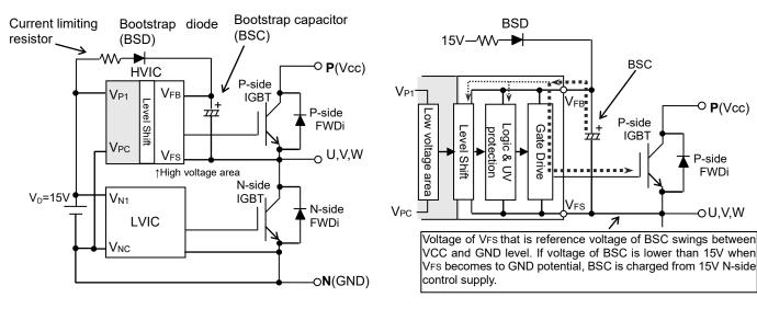
Fig.4-1-1 Bootstrap Circuit Diagram
