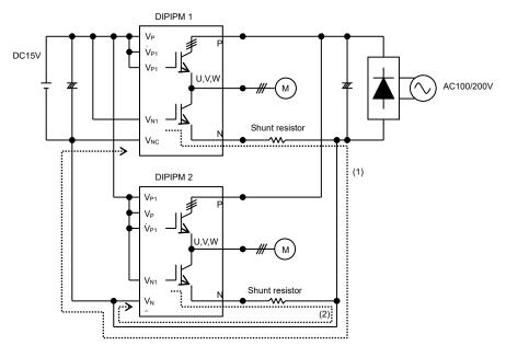
Fig.3-1-14 Parallel operation
