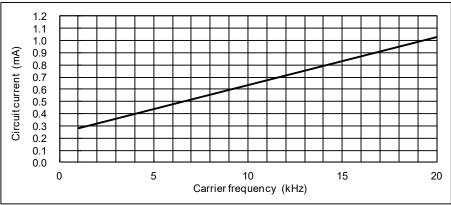
Fig.4-2-5 I<sub>DB</sub> vs. Carrier frequency for PSS10S51F6 (10A/600V))
