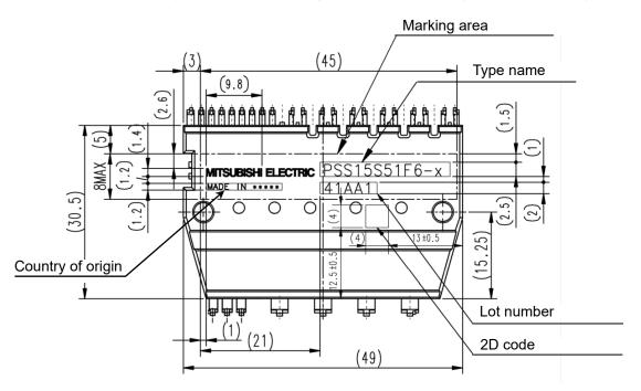
Fig.2-3-5 Laser marking view PSSxxS51F6 (Dimension in mm)
