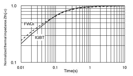
Fig.2-1-3 Typical transient thermal impedance (PSSxxS71F6)
