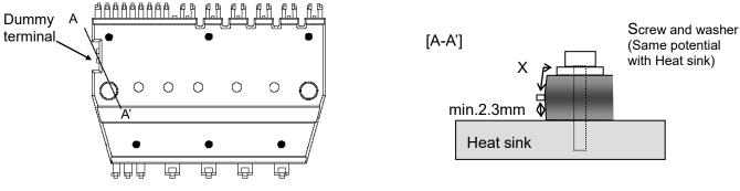
Fig.2-4-1 Creepage between dummy terminal and heat sink
