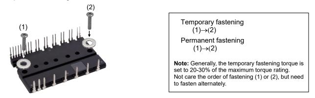
Fig.2-4-2 Recommended screw fastening order
