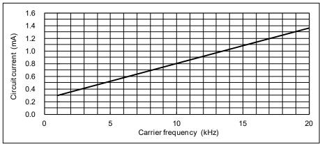
Fig.4-2-6 I<sub>DB</sub> vs. Carrier frequency for PSS15S51F6 (15A/600V))
