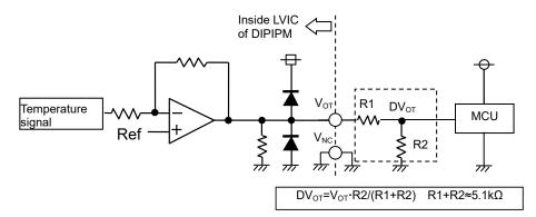
Fig.2-2-11  $V_{\text{OT}}$  output circuit in the case with high protection level
