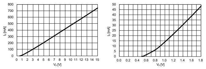
Fig.4-3-1 V<sub>F</sub>-I<sub>F</sub> curve for bootstrap Diode (The right figure is enlarged view)
