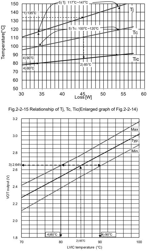
Fig.2-2-16 V<sub>OT</sub> output vs. LVIC temperature (Enlarged graph of Fig.2-2-12)
