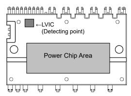
Fig.2-2-6 Temperature detecting point
