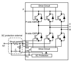
Fig.2-2-1 SC protecting circuit
