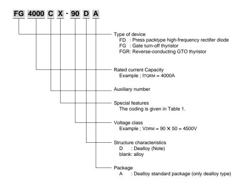
Note: Dealloy means without any alloying of the silicon wafer and metal disk.
