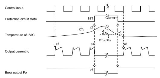
Fig.2-2-7 Timing Chart of OT protection
