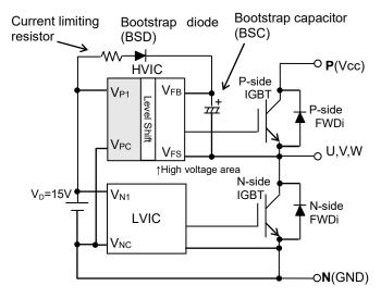
Fig.4-1-1 Bootstrap Circuit Diagram
