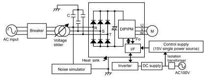
Fig.3-3-1 Noise withstand capability evaluation circuit
