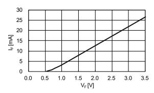
Fig.4-3-1 V<sub>F</sub>-I<sub>F</sub> curve for bootstrap Diode (rated current 5A~20A, the right figure is enlarged view)
