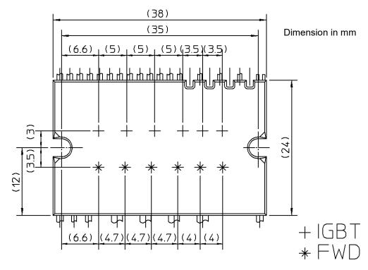
Fig.2-1-2 Power chip position
