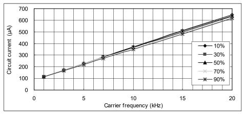
Fig.4-2-1 IDB vs. Carrier frequency for PSS05S92\*6-AG
