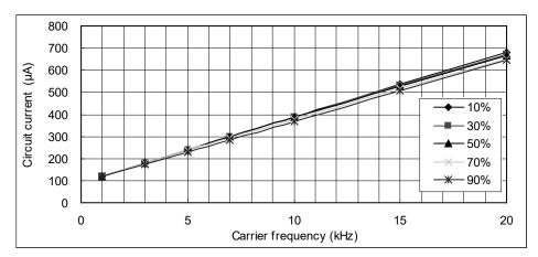
Fig.4-2-2 IDB vs. Carrier frequency for PSS10S92\*6-AG
