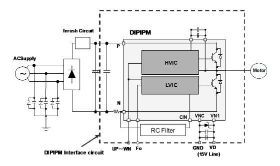
Fig.5-1-1 Demo board interface circuit
