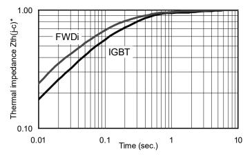
Fig.2-1-3 Typical transient thermal impedance
