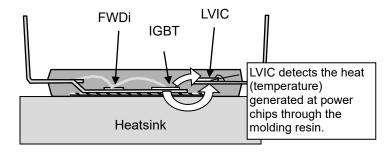
Fig.2-2-9 Thermal conducting from power chips
