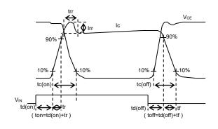
Fig.2-1-4 Switching time definition
