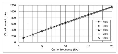
Fig.4-2-4 IDB vs. Carrier frequency for PSS20S92\*6-AG
