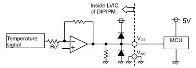
Fig.2-2-10 V<sub>OT</sub> output circuit
