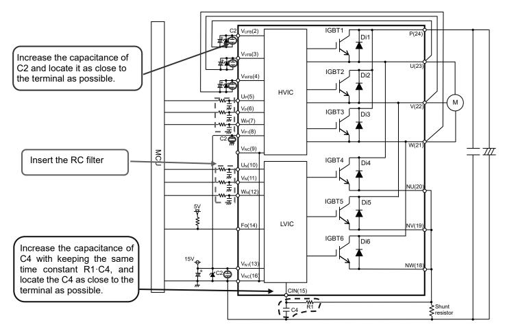
Fig.3-3-2 Example of countermeasures for inverter part
