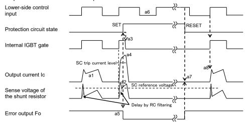
Fig.2-2-3 SC protection timing chart
