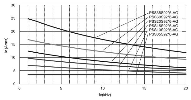
Fig.3-2-2 Effective current-carrier frequency characteristics
