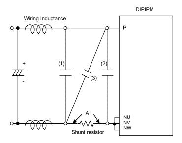
Fig.3-1-8 Recommended snubber circuit location
