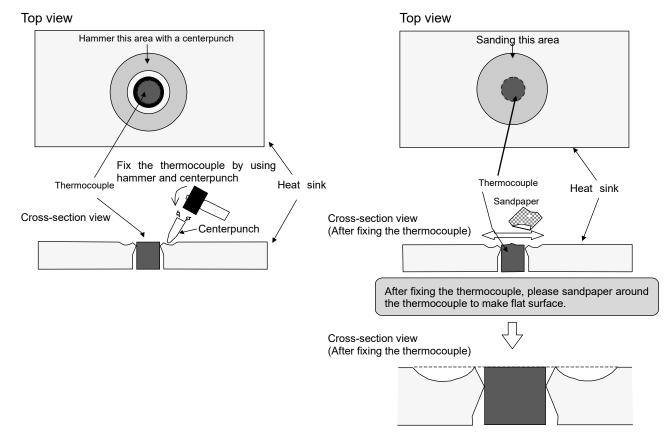
Fig. 3-2-5 Example of installation of thermocouple
