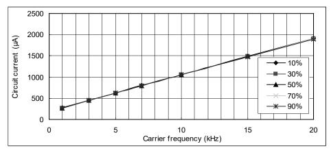
Fig.4-2-5 IDB vs. Carrier frequency for PSS30S92\*6-AG
