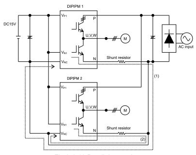
Fig.3-1-13 Parallel operation
