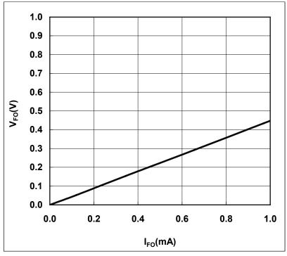
Fig.3-1-7 Fo terminal typical V-I characteristics ( $V_D=15V$ ,  $T_i=25$ °C)
