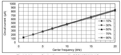
Fig.4-2-3 I<sub>DB</sub> vs. Carrier frequency for PSS15S92\*6-AG
