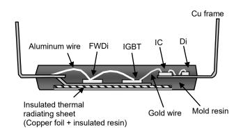
Fig.1-1-2 Internal cross-section structure
