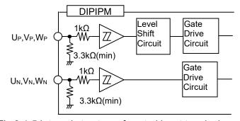
Fig.3-1-5 Internal structure of control input terminals
