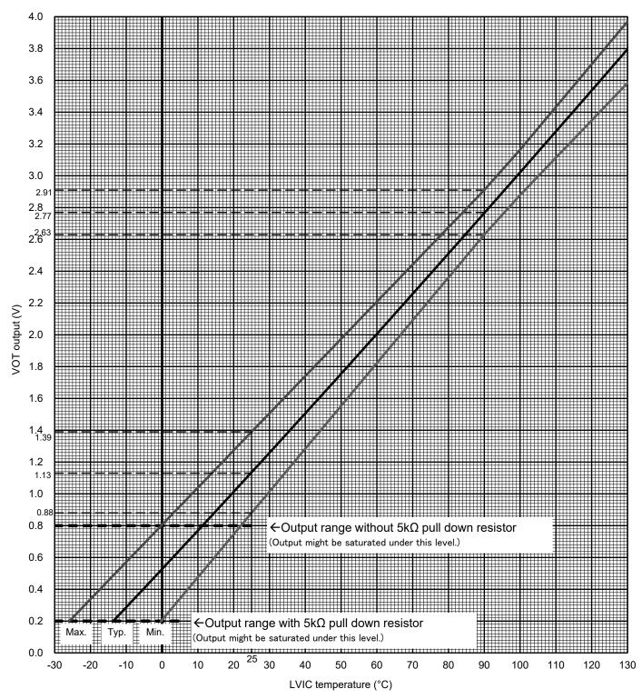
Fig.2-2-14 V<sub>OT</sub> output vs. LVIC temperature
