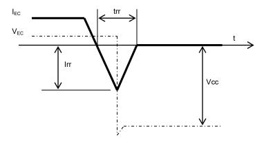
Fig.3-2-1 Ideal FWDi recovery characteristics curve
