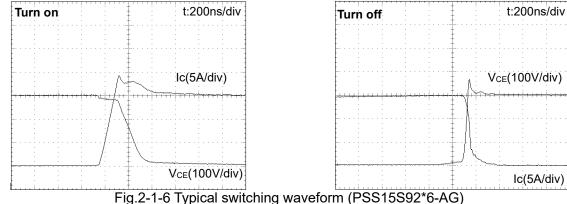
Conditions: V<sub>CC</sub>=300V, V<sub>D</sub>=V<sub>DB</sub>=15V, Tj=125°C, Ic=15A, Inductive load half-bridge circuit
