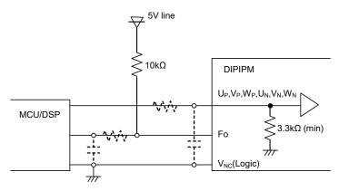
Fig.3-1-6 Control input connection
