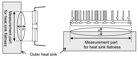
Fig.2-4-2 Measurement point of heat sink flatness
