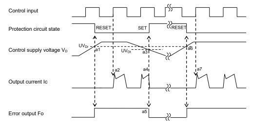
Fig.2-2-4 Timing chart of N-side UV protection
