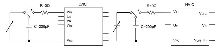
Fig.3-3-3 LVIC terminal Surge Test circuit
