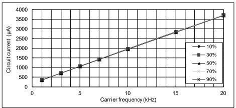
Fig.4-2-6 I<sub>DB</sub> vs. Carrier frequency for PSS35S92\*6-AG
