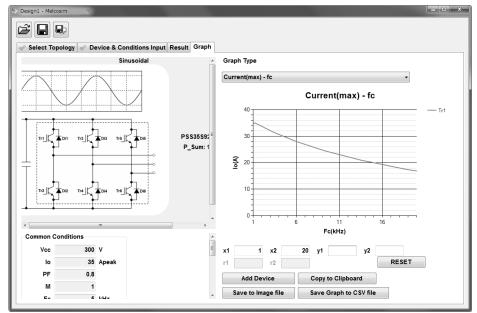
Fig.3-2-3 Loss simulator screen image
