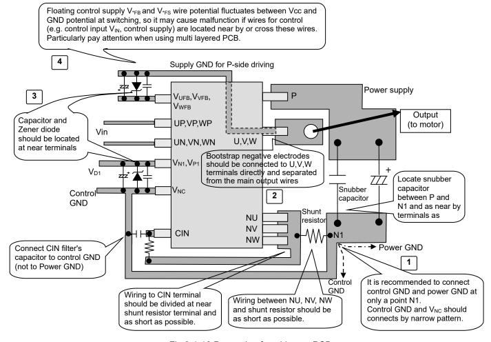
Fig.3-1-12 Precaution for wiring on PCB
