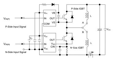
Fig.2-1-5 Evaluation circuit (inductive load)
