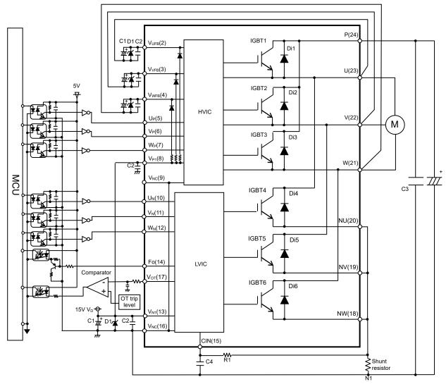
Fig.3-1-3 Interface circuit example with optocoupler
