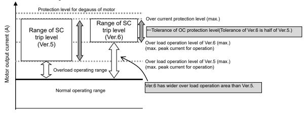
Fig.1-5-1 short circuit trip level
