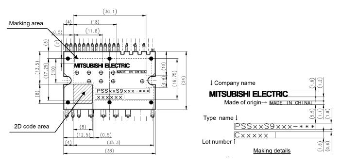
Fig.2-3-2 Laser marking view
