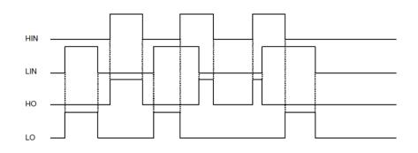
2. V<sub>CC</sub> (V<sub>BS</sub>) Supply Under Voltage (UV) Lockout Timing Diagram
