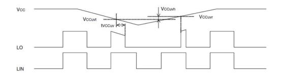
If V<sub>CC</sub> supply voltage drops below UV trip voltage (V<sub>CC</sub>uvt) for V<sub>CC</sub> supply UV filter time, HO output signal is shut down. And then, if V<sub>CC</sub> supply voltage rises over UV reset voltage, HO will return to the usual operation mode.
