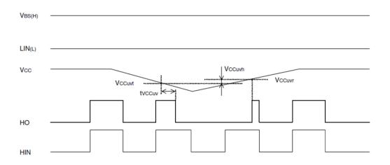
If  $V_{BS}$  supply voltage drops below UV trip voltage ( $V_{BS}uvt$ ) for  $V_{BS}$  supply UV filter time, HO output signal is shut down. And then, if  $V_{BS}$  supply voltage rises over UV reset voltage, HO will respond to the next active HIN signal( $L \rightarrow H$ ).
