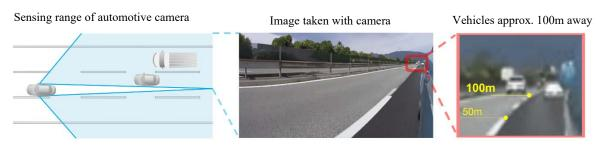
Camera-monitoring system for mirrorless car
