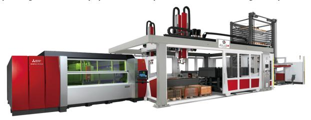
Sheet metal laser processing machine
