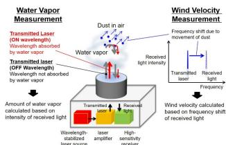
Demonstration water vapor DIAL and wind LIDAR
