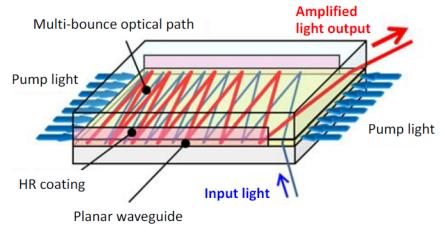
Structure of planar waveguide laser amplifier
