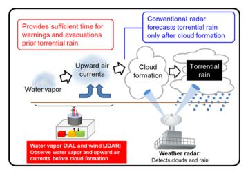
The new system, which is based on a conventional wind LIDAR that Mitsubishi Electric released on May 28, 2014, has been enhanced for the measurement of water atmospheric vapor. It transmits laser beams from the ground to simultaneously measure the amount and distance of water vapor as well as the speed and direction of wind.
