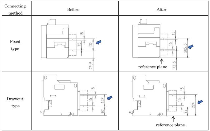
Above figures are on the side view of the horizontal terminal of AE630-SW, AE1000-SW, AE1250-SW, AE1600-SW.
