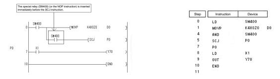
(2) If the immediately preceding instruction meets the conditions described in 2.Condition above, inserting the special relay SM400 (or NOP instruction) is not required. Therefore, use the existing program as shown below.
