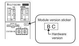
The sticker of the A1SJ71UC24-R2, A1SJ71UC24-PRF, and A1SJ71UC24-R2-S2 is placed as follows:
