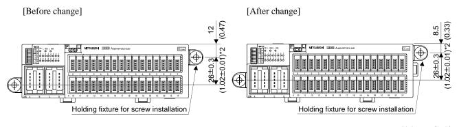
\*2: The length needed for screw installation (mounting pitch) has not been changed.
