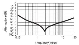
Fig.2. Damping characteristics of noise filter
