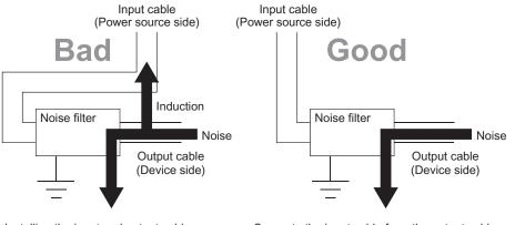
Installing the input and output cables together will cause noise induction.
