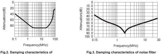
noise filter for AC powered main unit
