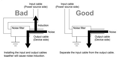
Fig.4. Precautions on noise filter
