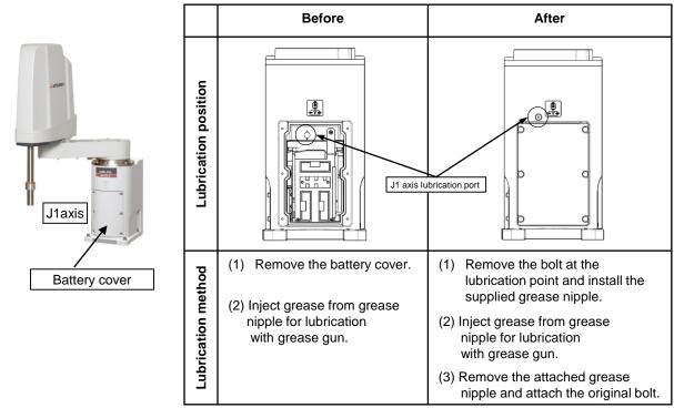
(2) Along with this change, the contents of "Section 5.3.6 Lubrication" in "5. Maintenance and inspection" of "Instruction manual BFP-A 8864, BFP-A 3314" will be changed.
