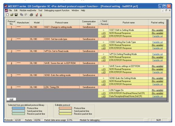
Configure protocol No.2 and No.3 so that the data to be sent will be read from the following CPU devices and set into a send packet.
