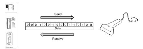
(1) When the A1SJ71UC24-R2/R4/PRF sends data to an external device
