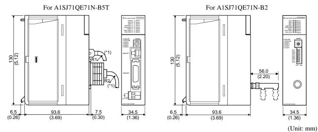
\*1: The bending radius near the connectors (reference value: R1, R2) should be four times larger or more than the cable's external diameter when connecting the communication cable.
