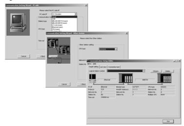
\* On MX Component, all supported communication routes are set by this communication setup utility. The logical station numbers are managed together as one regardless of the communication routes.
