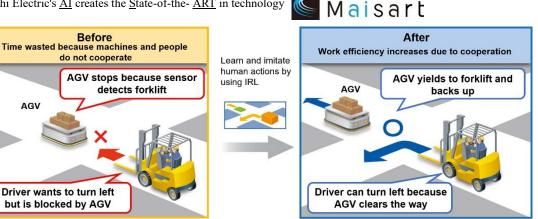
Example of cooperative AI deployed in AGV
