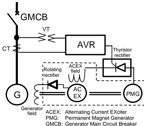
Fig. 1 Brushless excitation system configuration
