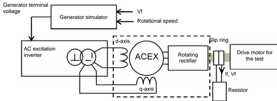
Fig. 12 Circuit for the assembly test
