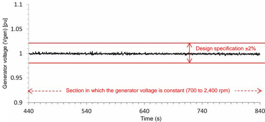
Fig. 14 Test results of the generator terminal voltage control
