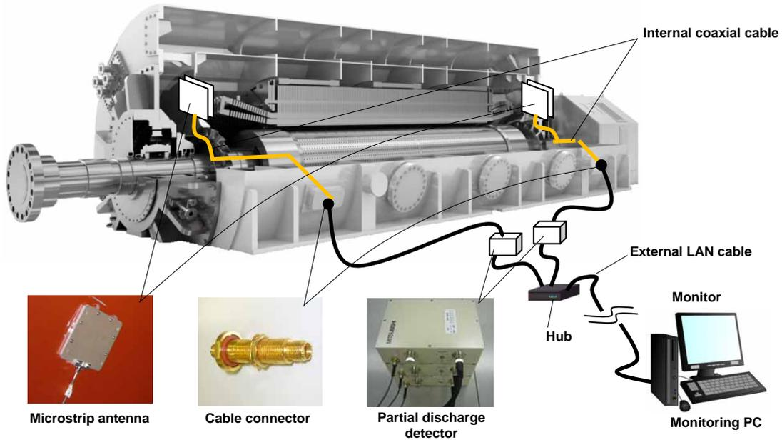
Fig. 5 Schematic view of the configuration of the online partial discharge monitoring system
