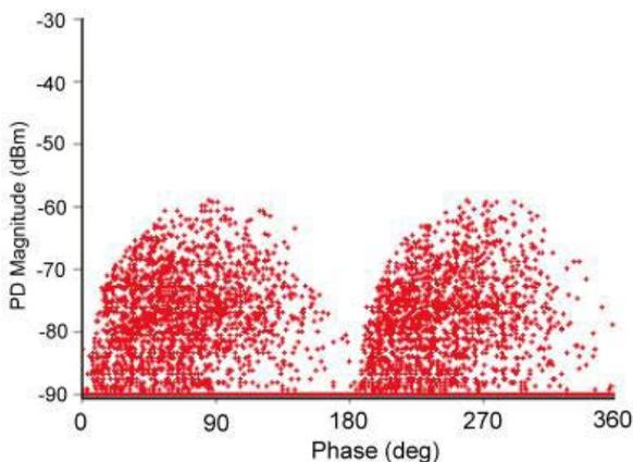
Fig. 6 PD phase characteristics (typical measurement result)
