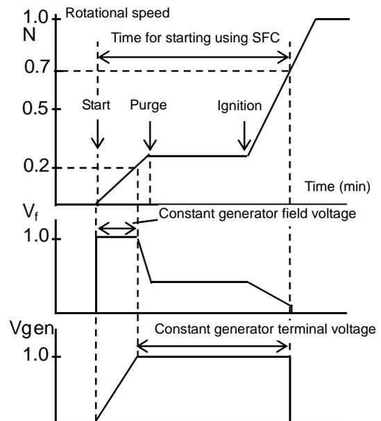
Fig. 5 Generator field voltage and terminal voltage when a GT is started using an SFC (example)
