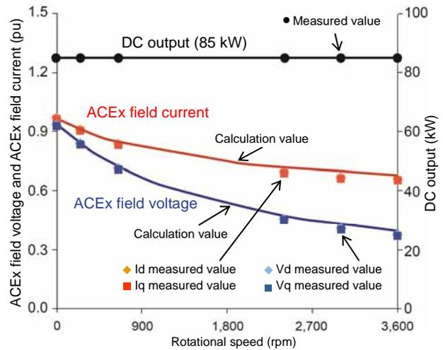
Fig. 9 Load characteristics of the AC field winding brushless exciter
