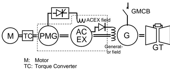
Fig. 3 Motor starting system
