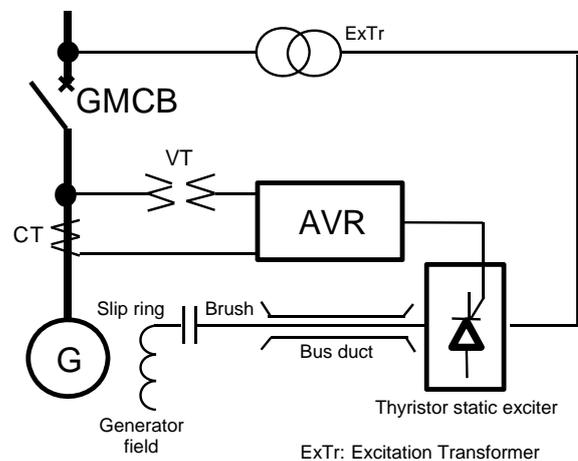
Fig. 2 Thyristor static excitation system configuration
