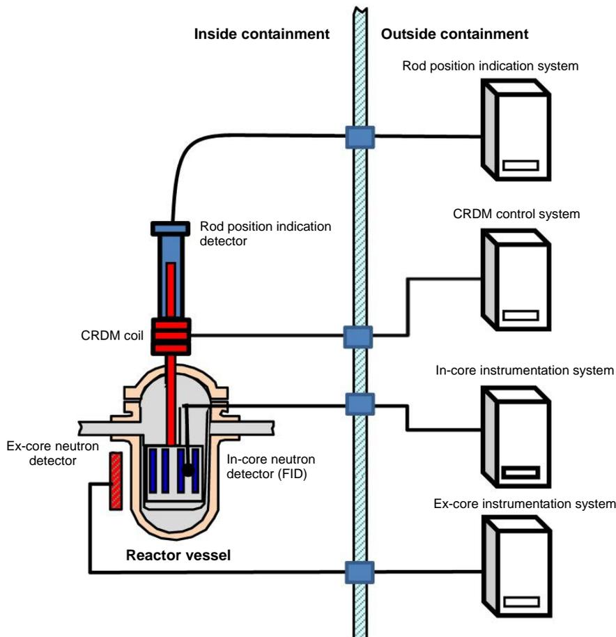
Fig. 3 Reactor I&C systems
