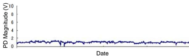
Fig. 7 PD magnitude trend (typical measurement result)
