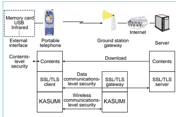
Fig. 1 W-CDMA mobile mobile-phone data security technology
