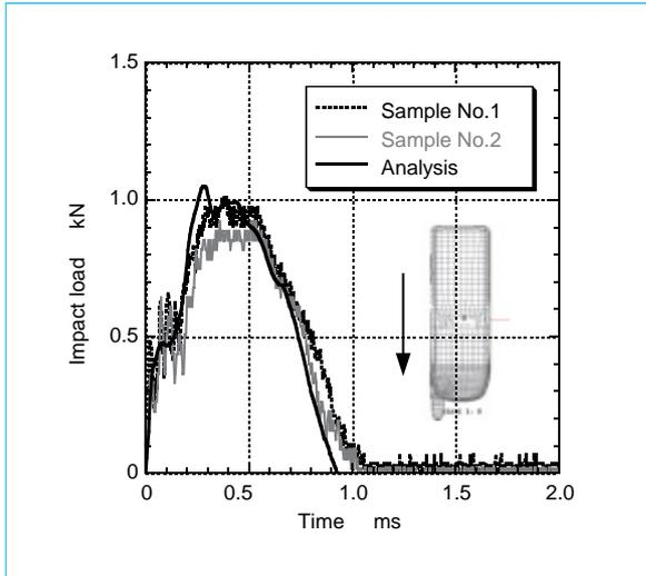
Fig. 2 Time history waveform of impact load
