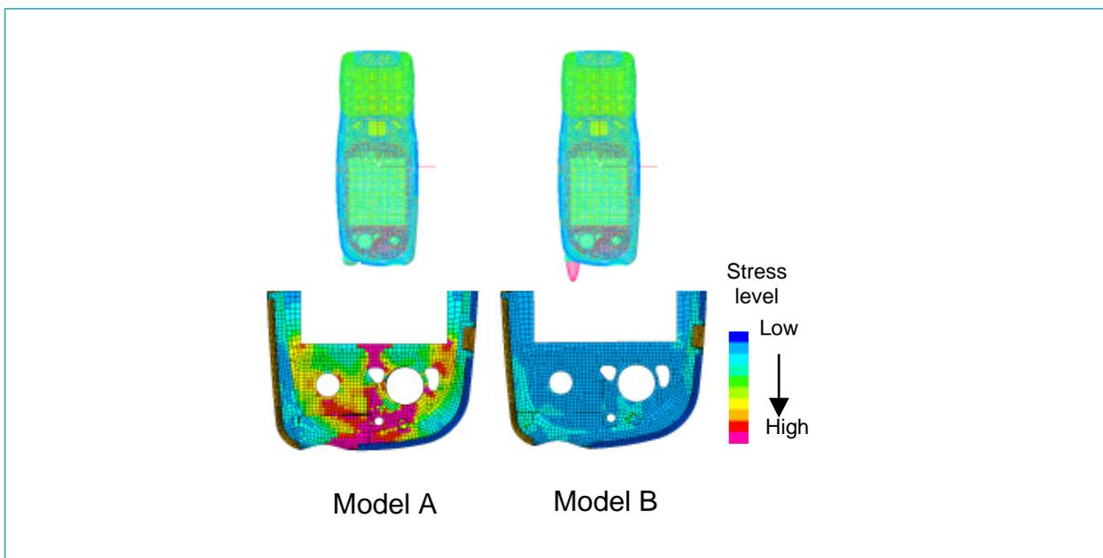
Fig. 3 Stress distribution around the top of the Mg chassis
