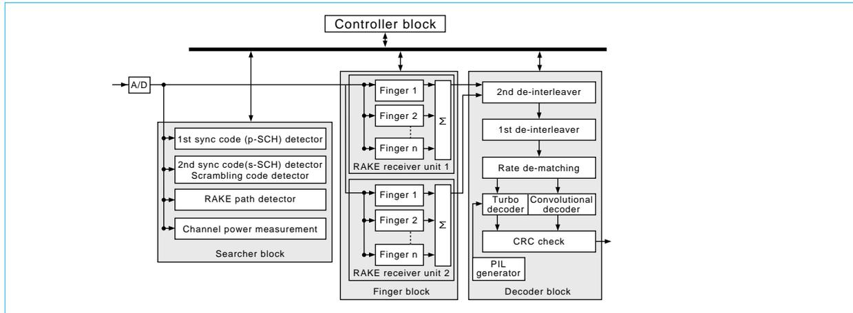
Fig. 2 Block diagram of the digital baseband demodulator
