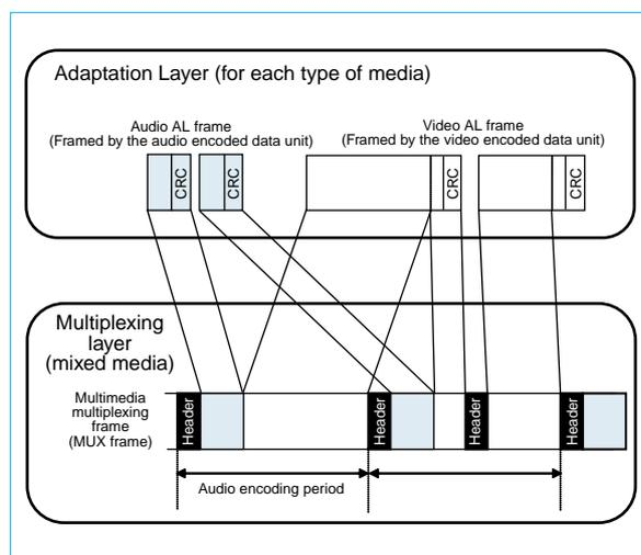
Fig. 3 Multiplex Format in H.223
