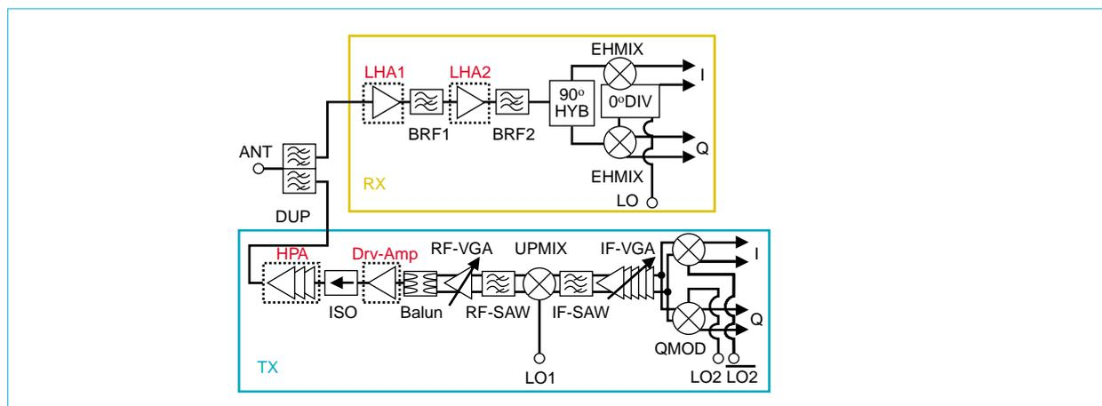
Fig. 1 Block diagram of RF section
