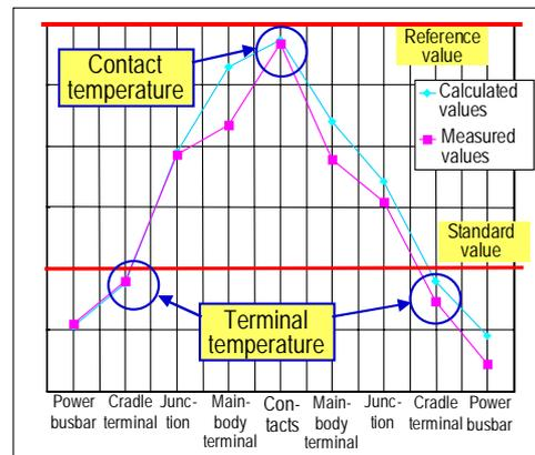
Fig. 3 Results of calculations and actual measurements on thermal circuit network
