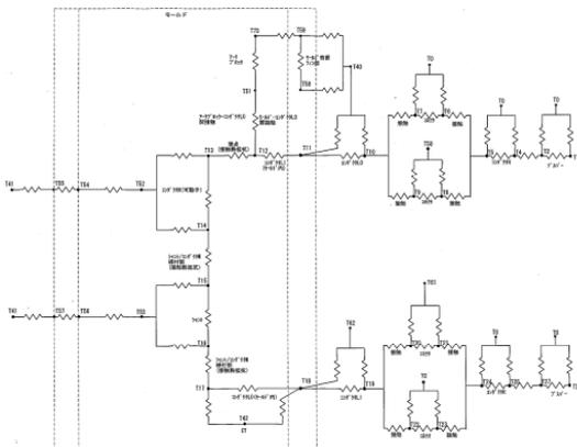
Fig. 2 Thermal circuit network of AE2000-SWA
