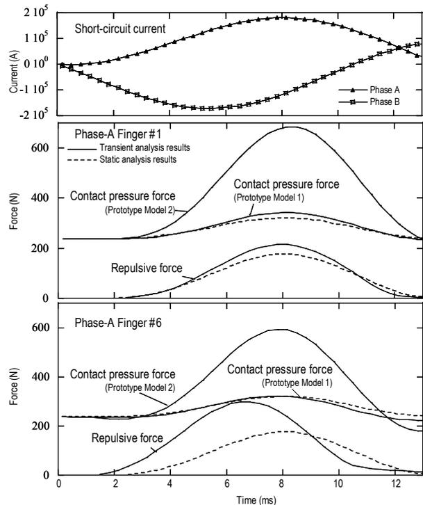
Fig. 5 Contact pressure and repulsive force of Fingers #1 and #6
