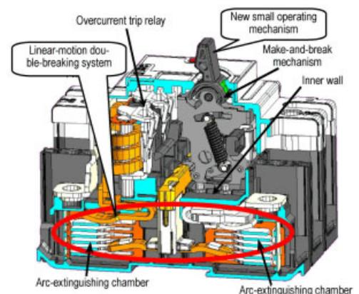
Fig. 2 Internal construction of NF100-HRU
