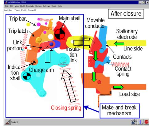
Fig. 7 ACB in the ON position & in a discharged state
