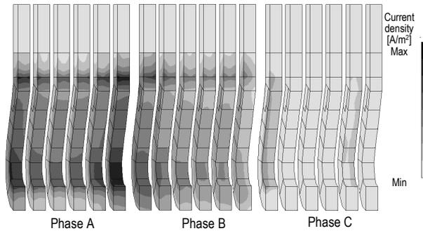
Fig. 4 Current density distribution among finger conductors (6 ms after commencement of energization)
