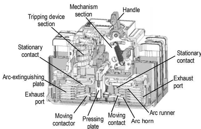
Fig. 1 New low-voltage circuit breaker with linear-motion double-breaking system
