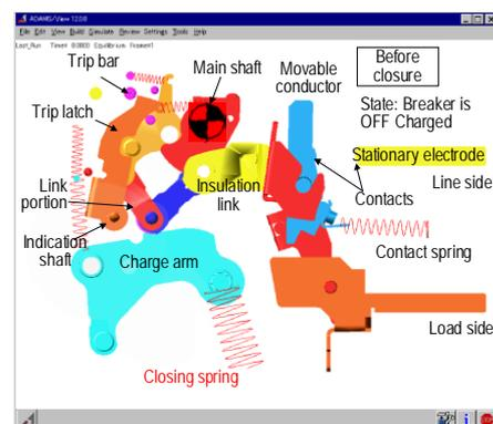
Fig. 5 ACB in the OFF position & in a charged state
