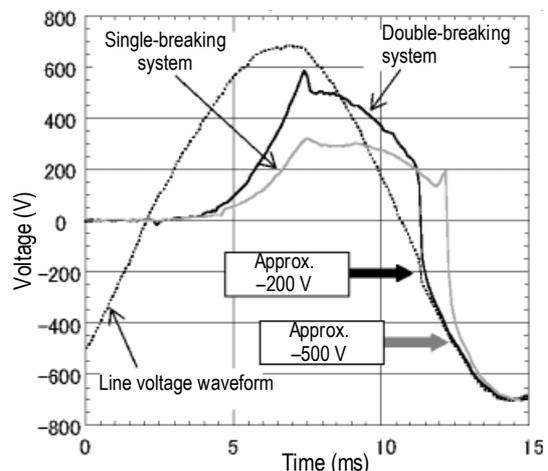
Fig. 2 Restriking voltages of double-breaking system and single-breaking system
