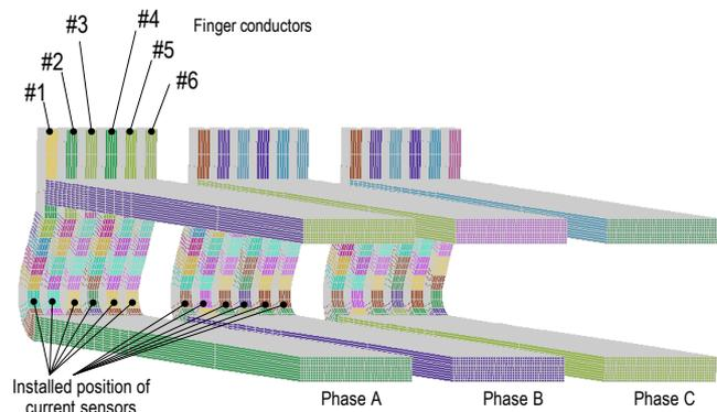
Fig. 2 Mesh model of the main circuitry of AE4000-SWA
