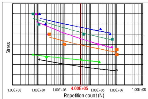
Fig. 8 S-N curves of candidate materials for mechanisms
