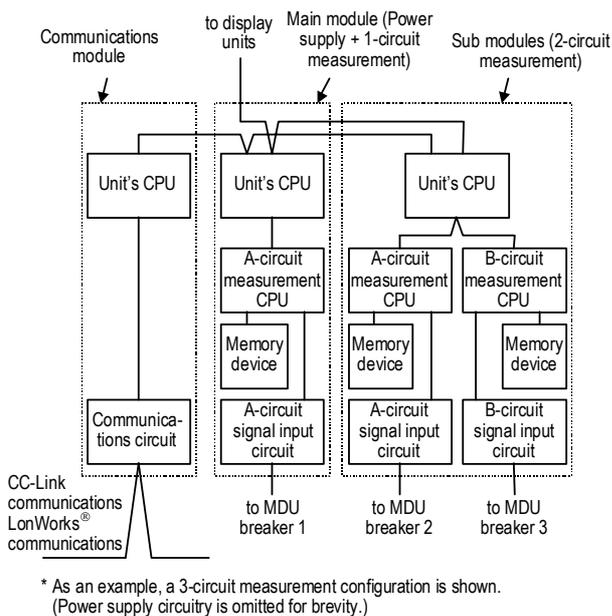
Fig. 2 Block diagram of MDU2
