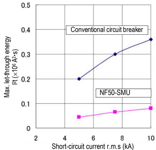
Fig. 4  $I^2t$  let-through characteristics comparison (AC 220 V)
