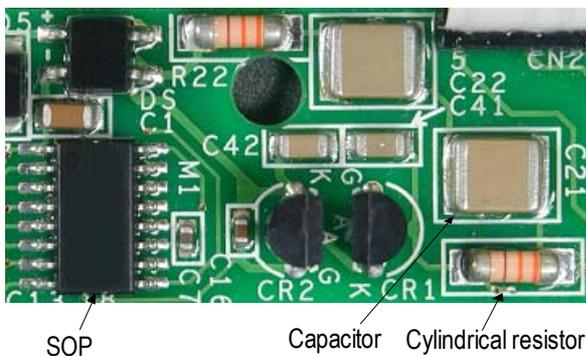
**Fig. 1 Example of printed circuit board in low-voltage circuit breaker**
