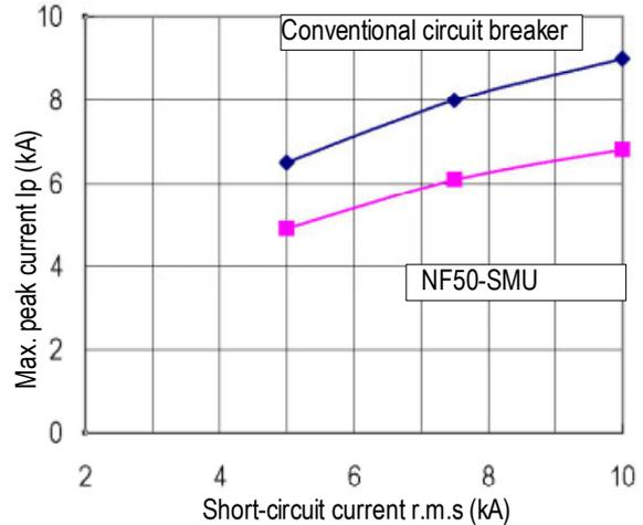
Fig. 3 Current-limiting characteristics comparison (AC220V)
