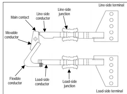
Fig. 1 Conductor structure of air circuit breaker
