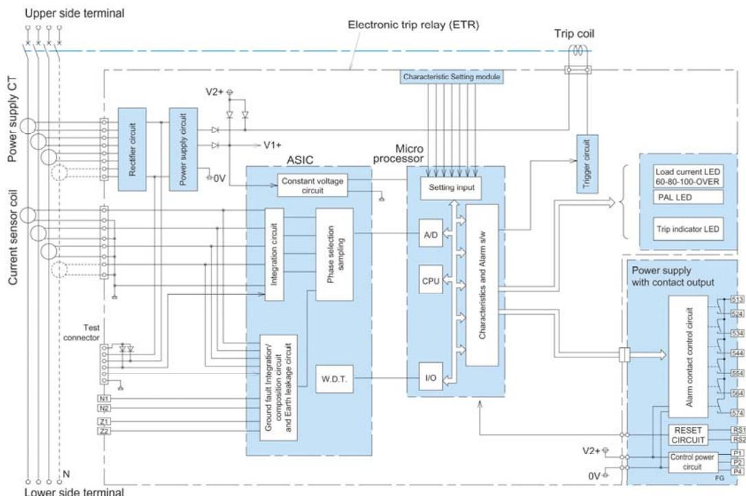
Fig. 1 Electronic trip relay circuit diagram
