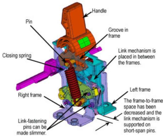
Fig. 3 Parts layout of new operating mechanism
