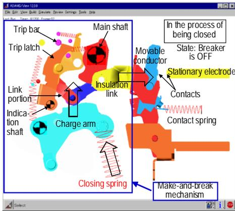
Fig. 6 ACB in the process of being turned ON
