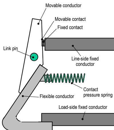
Fig. 1 Cross-sectional view of the construction of ACB main circuitry
