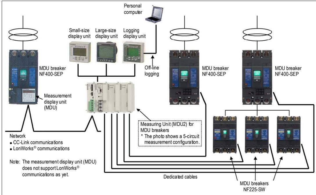
Fig. 4 Example of connection of MDU Breaker and MDU2
