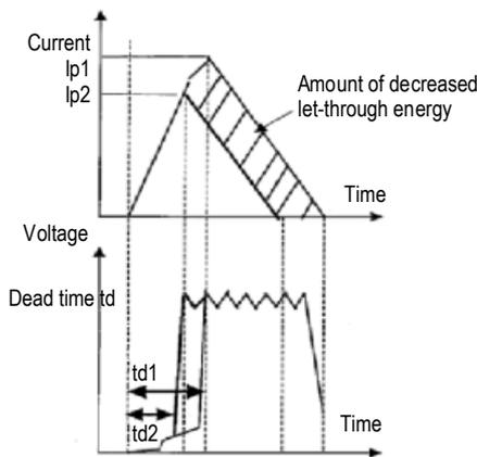
Fig. 2 Current-limiting waveform
