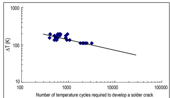
**Fig. 2 Solder crack lifetime of cylindrical resistor**
