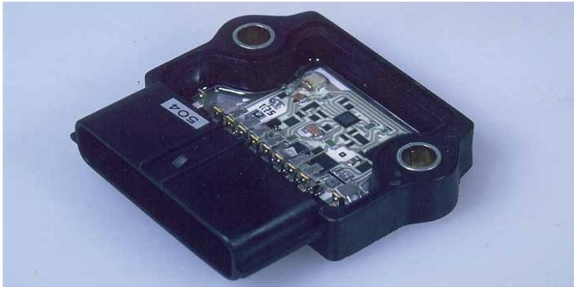
The ionic current detection module.
