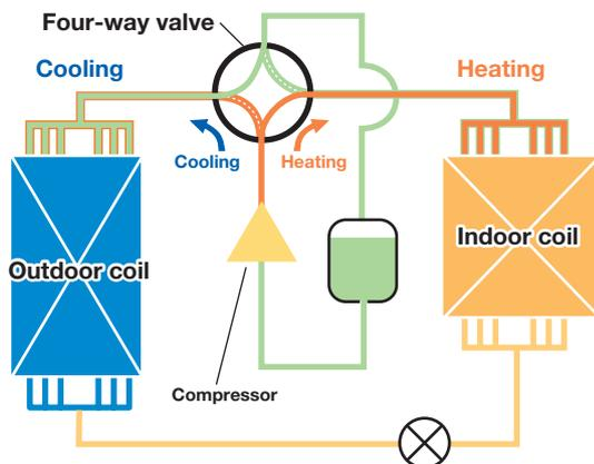
Reduce power consumption with high efficient refrigerant cycle
