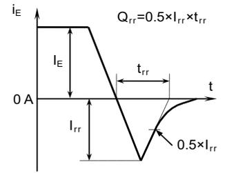
$t_{rr}$ ,  $Q_{rr}$  characteristics test waveform
