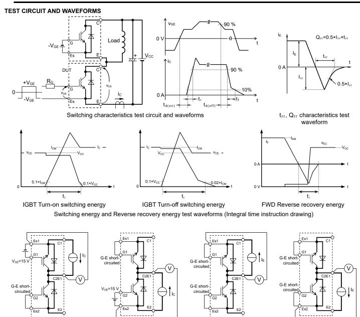
V<sub>CEsat</sub> characteristics test circuit
