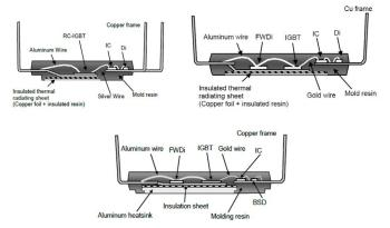
Figure 3: Internal structure (clockwise): SLIMDIP™, Super Mini DIP-IPM™ and Large DIPIPM™
