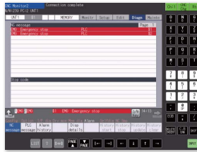
Alarm screen (CNC monitor 2)
