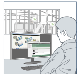
Work reports and equipment pictures saved in multiple (up to 50) GOTs can be displayed collectively on a PC for data management
