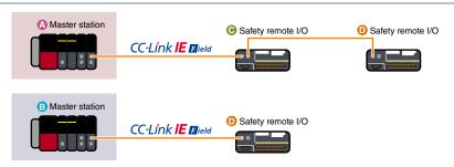
(a) Safety protocol versions: 1 and 2 Master station (safety CPU module): firmware version 29 or later (master module RJ71GF11-T2): firmware version 70 or later
