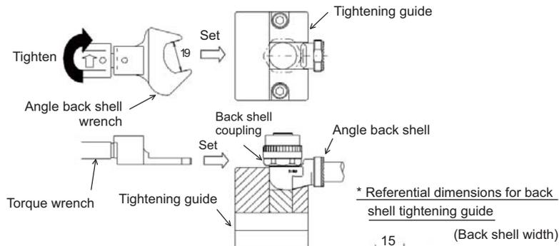
(Note) To change the back shell angle, adjust the toothing position of the plug shell and back shell.
