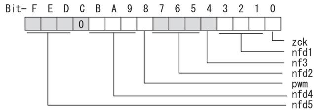
**bit F-D : nfd5 Depth of Notch filter 5**
