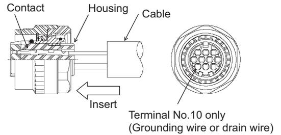
(Note) Before inserting the contact, check that the clamp nut, cable clamp, bushing and back shell is inserted.
