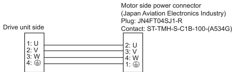
1. The main circuit cable must be manufactured by the user.
