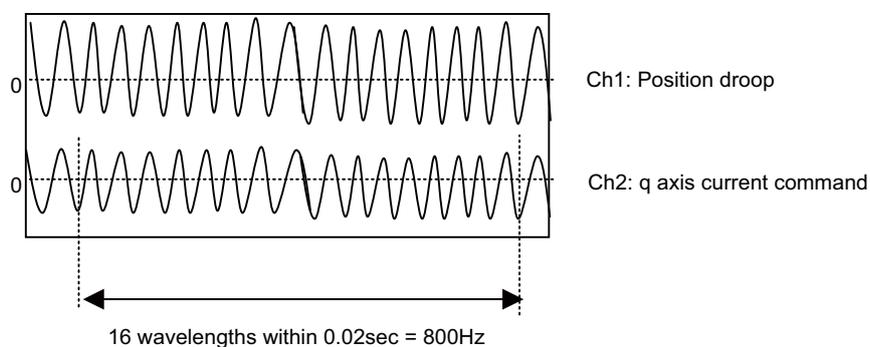
Set 800 to SP038 and XXX0 to SP034. Measure position droop and current command at this time, and adjust notch filter's frequency and depth so that the position droop is within standard range.
