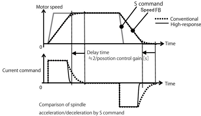
**【#13095】 SP095 VIAX Lead compensation scale during high-response acceleration/deceleration**
