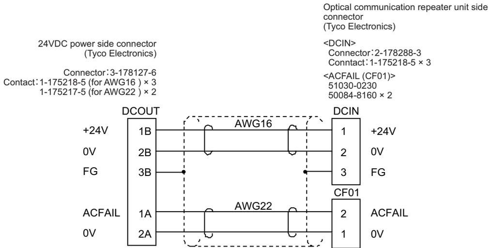
Appendix 1-2-4 Servo / tool spindle detector cable
