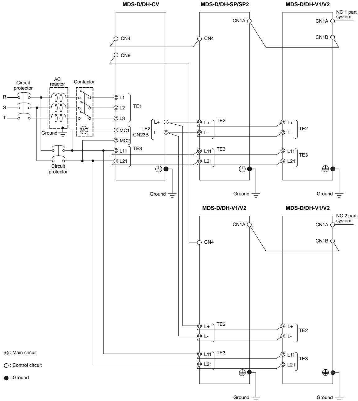
1. If the two NC communication bus systems include a spindle drive unit, connect the power supply unit's CN4 connector to the CN4 connector of the largest-capacity spindle drive unit. If there is no spindle drive unit, connect to the unbalance-axis servo drive unit.
