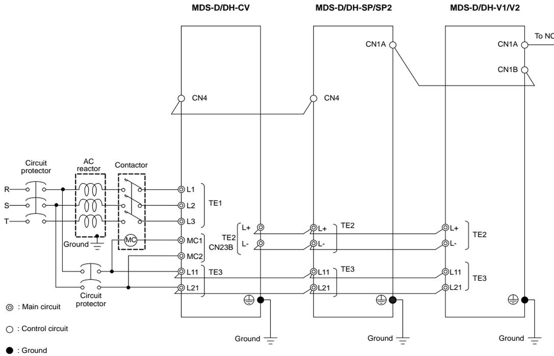
1. The power supply unit is a power supply regenerative type converter; an AC reactor is surely installed in the power supply line.
