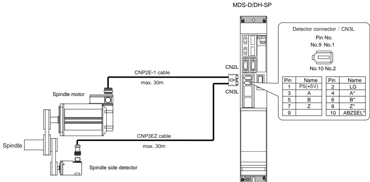
(Note) Confirm that the gear ratio (pulley ratio) of the spindle end to the detector is 1:1. Use a timing belt for connecting.
