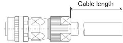
$$\begin{aligned} \text{Cable length after cutting} &= 35 \pm 0.5 \text{mm for CM10-SPxxS-x(D6)} + \text{Cable length} \\ &= 35 \pm 0.5 \text{mm} + \text{Cable length} \end{aligned}$$
