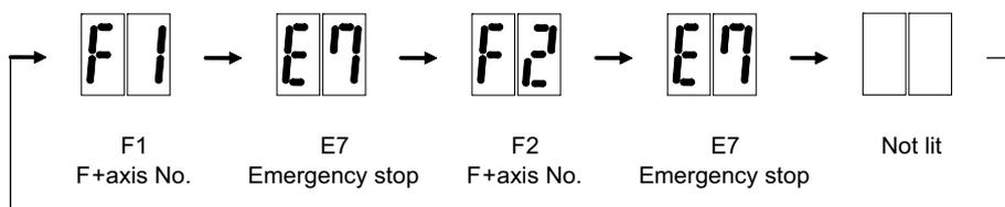
Normal drive unit LED display at NC power ON (for 1st axis)
