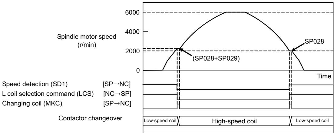
Spindle motor coil changeover control
