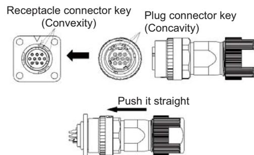
\* To remove, rotate the coupling and pull out to straight.
