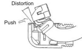
Turn the form of the ground clip back to normal and position it for the receptacle case as shown in the right figure.
