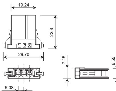
**Power supply unit connector for CN23 (Contactor control output / external emergency stop)**
