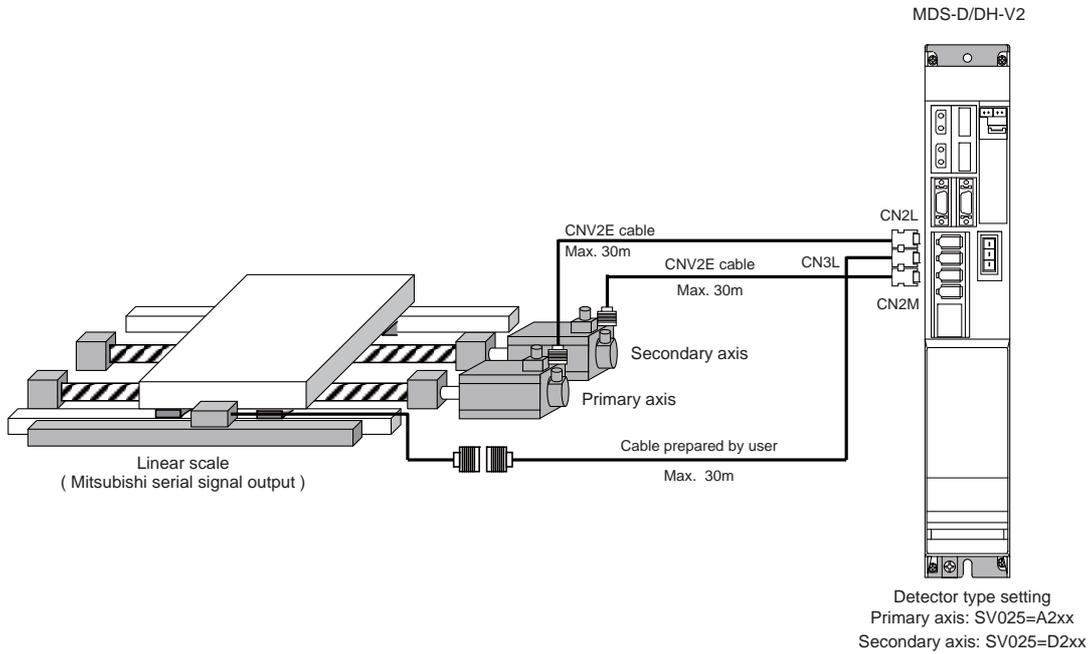
**(4) Connecting Mitsubishi serial signal output linear scale (when using two units of MDS-D/DH-V1)**
