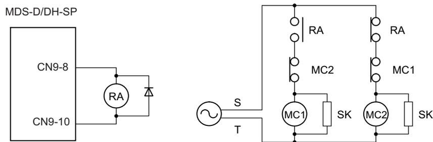
Coil changeover relay control circuit
