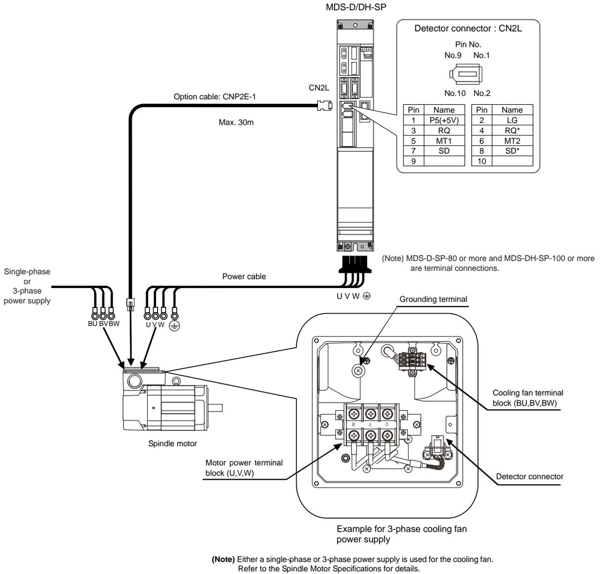
**CAUTION** For a 3-phase cooling fan, when the phase sequence of the 3-phase power supply is connected reversely, its cooling capacity degrades due to the reversed rotation direction. Make sure the air blowoff direction.
