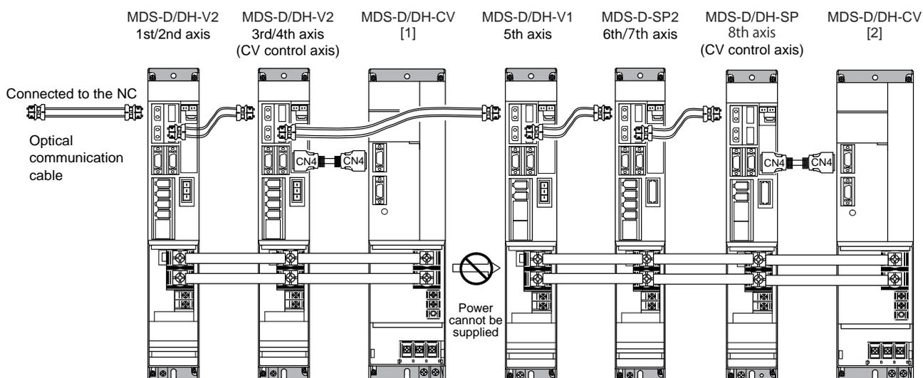
Connections when using two power supply units within a single NC communication bus system
