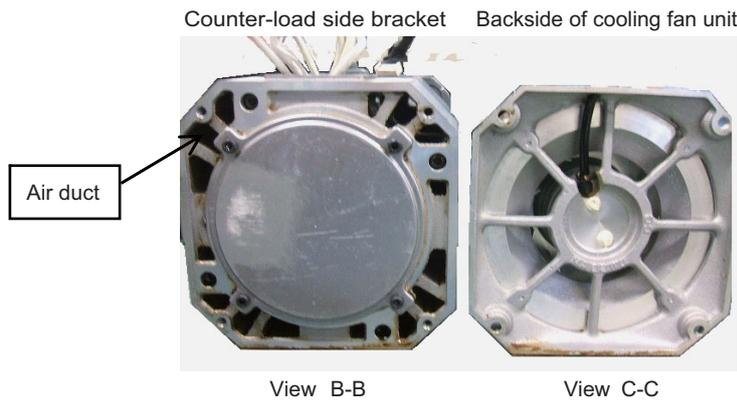
(b) Clean up the inner part of the fan case and the air duct of the spindle motor body
