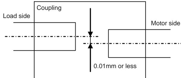
Also note that the motor side ball screw bearing must be locked so that to avoid the thrust load on the motor shaft due to expansion and contraction of the ball screw.
