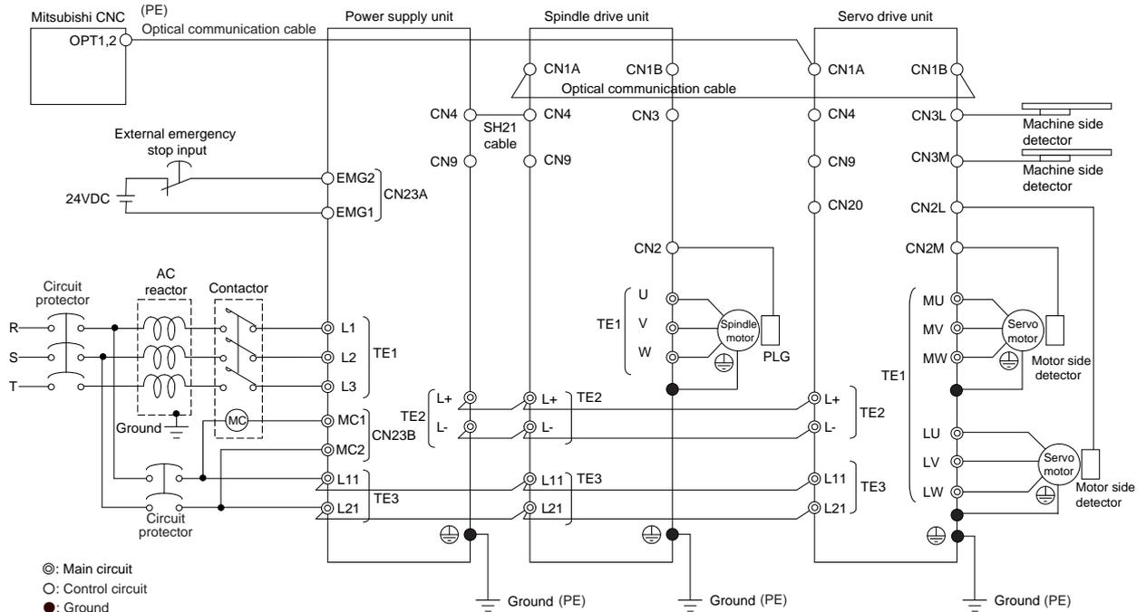
(Note 1) The total length of the optical communication cable from the NC must be within 30m and the minimum-bending radius within 80mm.
