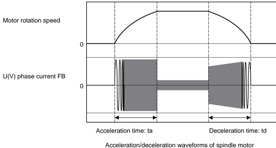
When acceleration/deceleration time does not match the theoretical value (an error rate 15% or more), check the following items.
