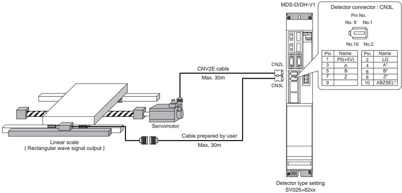
**(4) Connecting the linear scale (for SIN wave signal output)**
