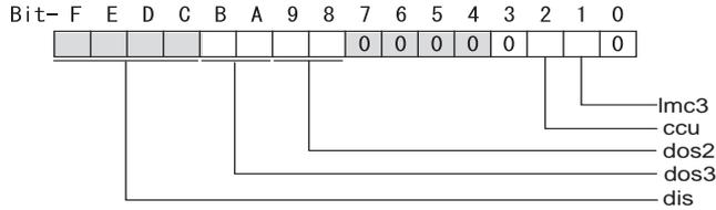
**bit F-C : dis Digital signal input selection**
