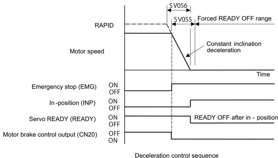
**【#2255】 SV055 EMGx Max. gate off delay time after emergency stop**
