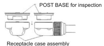
Confirm that the space between the receptacle case assembly and the POST BASE is within 1mm. Regarding POST BASE for inspection, contact with the sales department of the manufacturer below.
