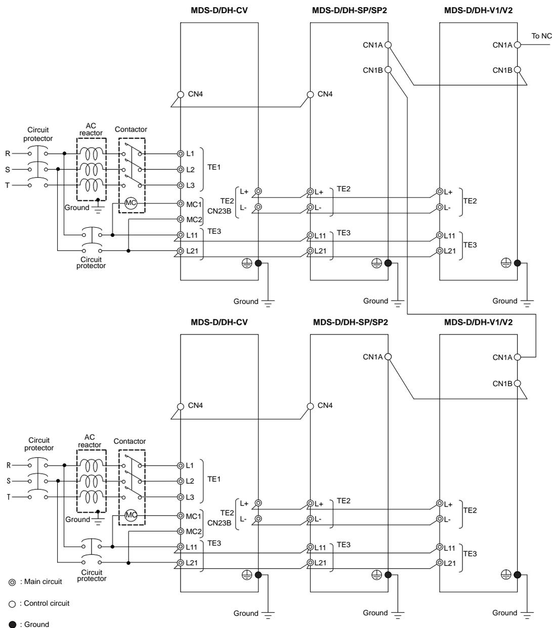
1. An AC reactor and circuit protector are required for each power supply unit.
