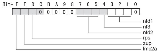
**bit F : lmc2a Lost motion compensation 2 timing**
