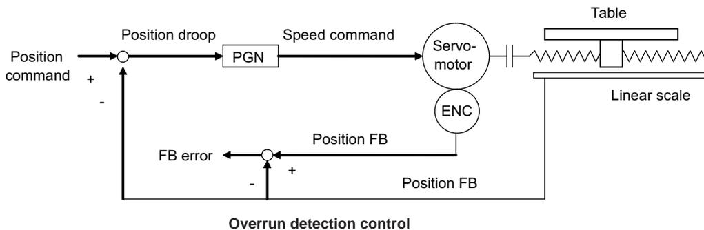
**【#2254】 SV054 ORE Overrun detection width in closed loop control**
