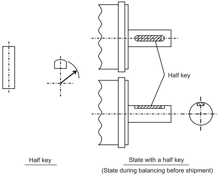
However if a full key is attached instead (See Figure 9 below), spaces that need balancing are generated when a fitting such as a gear, pulley and coupling is installed. Therefore take into consideration these spaces during the balancing of each fitting, or carry out balancing with the fittings attached to the motor.
