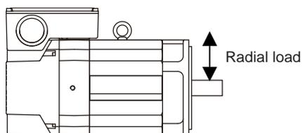
(Note) The load point is at the one-half of the shaft length.
