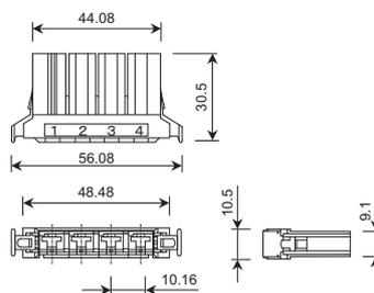
**Connector for motor brake control output**
