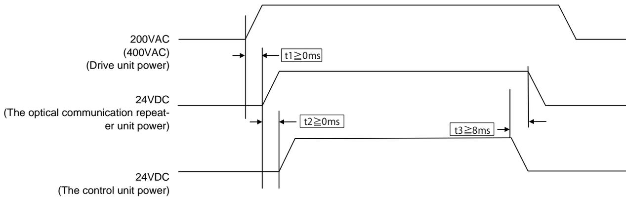
t1: Time lag between the power-ON of the drive unit and the optical communication repeater unit
