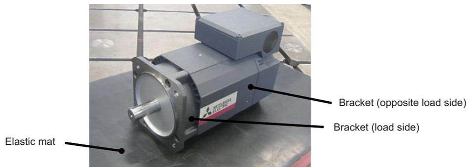
How to measure motor vibration
