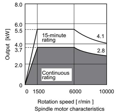
$$P_o = (\text{Short-time rated output}) \times 1.2 = 5500 \times 1.2 = 6600 \text{ [W]}$$
