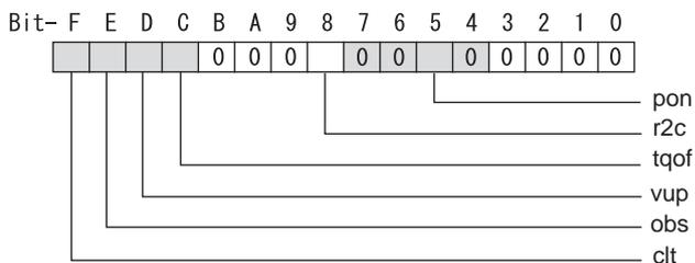
**bit F : clt Spindle monitor load inertia ratio**
