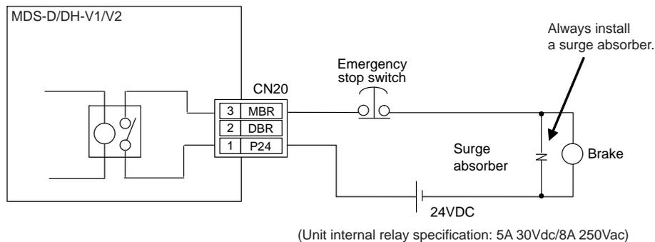
1. Always install a surge absorber near the motor's brake terminal to eliminate noise and protect the contacts.
