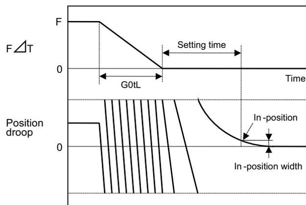
$$\text{Settling time (ms)} = \frac{10^3}{\text{PGN1}} \cdot \ln \left[ \frac{\frac{F \times 10^6}{60 \times \text{G0tL} \times \text{PGN1}^2} \times \left[ 1 - \exp \left[ -\frac{\text{PGN1} \times \text{G0tL}}{10^3} \right] \right]}{\text{INP}} \right]$$
