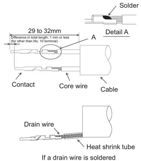
**(5) Inserting the contact**
