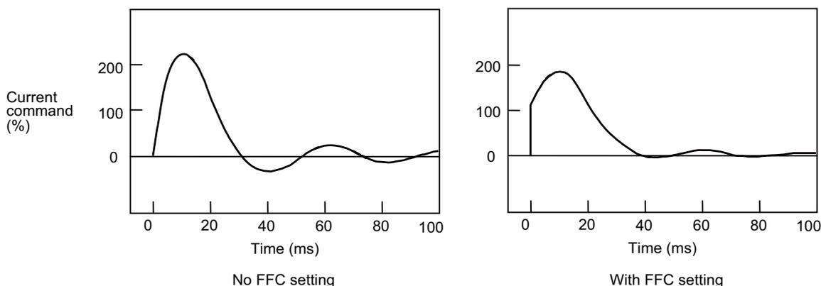
Acceleration rate feed forward gain means that the speed loop gain during acceleration/deceleration is raised equivalently. Thus, the torque (current command) required during acceleration/deceleration starts sooner. The synchronization precision will improve if the FFC of the delayed side axis is raised between axes for which high-precision synchronous control (such as synchronous tapping control and superimposition control).
