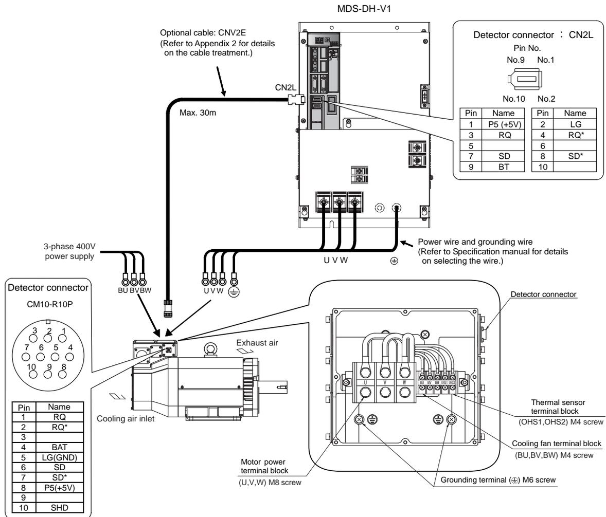
1. For a 3-phase cooling fan, when the phase sequence of the 3-phase power supply is connected reversely, its cooling capacity degrades due to the reversed rotation direction. Make sure the air blowoff direction.
