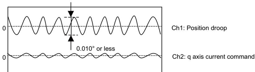
[2] When satisfactory accuracy is not secured, increase SP008 (VGN2) by 10 increments and adjust so that the accuracy level meets the standard. Note that the maximum setting value is 150 x [inertia ratio].
