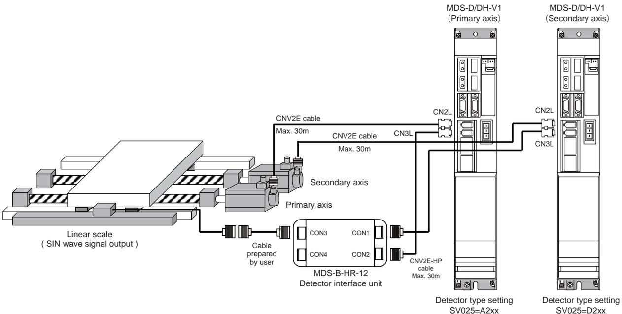
**(3) Connecting Mitsubishi serial signal output linear scale (when using MDS-D/DH-V2)**
