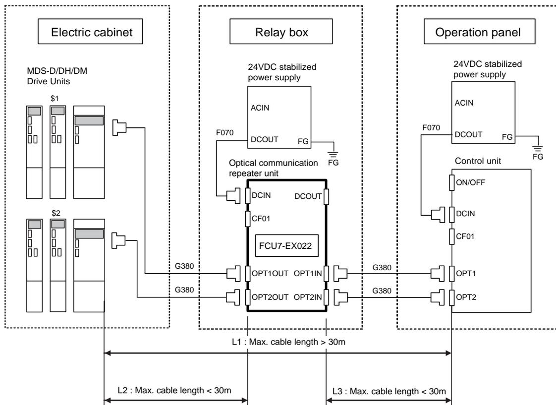
L1: Distance between the drive unit and the control unit.
