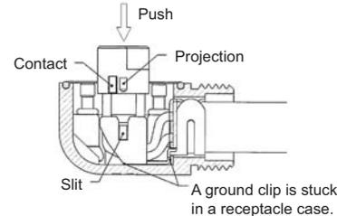
Adjust the projection of receptacle housing to the slit of the receptacle case and push in until it is fixed to the case.
