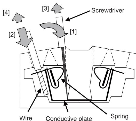
1. Connection of a cable is restricted to one to one spring.
