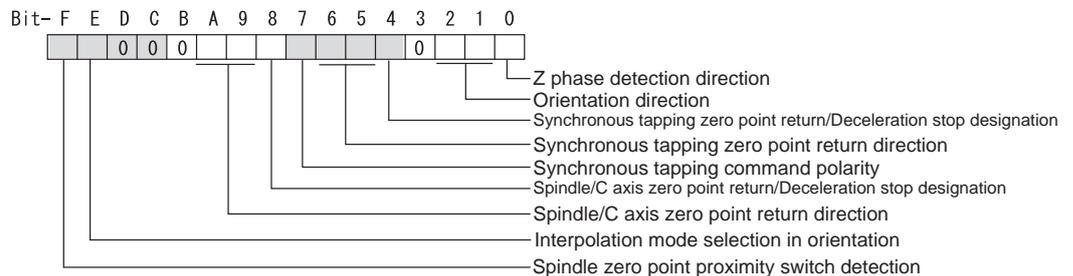
**bit F : Spindle zero point detection with contactless switch**
