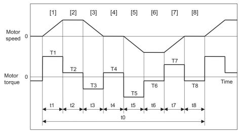
Fig. 1 Continuous operation pattern
