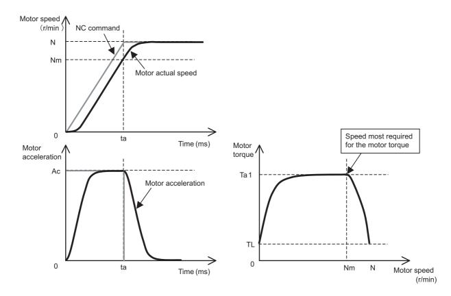
Fig.2 Speed, acceleration and torque characteristics when using the NC command linear acceleration/deceleration pattern + servo SHG control
