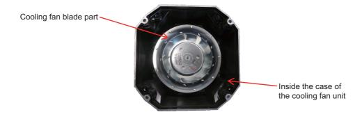
[2] Clean up the inside of the cooling fan unit and the cooling air vent.Wipe dirt off the inside of the cooling fan unit and the cooling air vent using wastes, etc.
