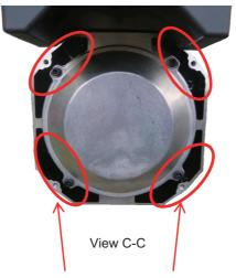
Motor frame's air ducts (cleaning points)
