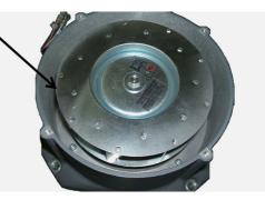
[5] Use the cleaning jigs to clean the air ducts of the spindle motor body.
