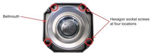
Cooling fan unit (before the bellmouth is removed)
