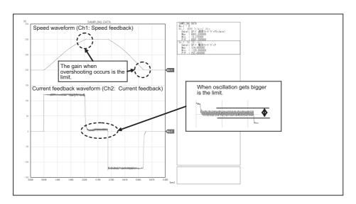
(Example)As the closest value should be selected from the standard setting range shown below, set 47 to SP001 when the limit gain is 55.
