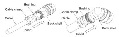
(Note) After the Bushing insert, confirm that cable position should be inside of Bushing.
