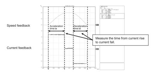
Acceleration/deceleration characteristics of spindle motor
