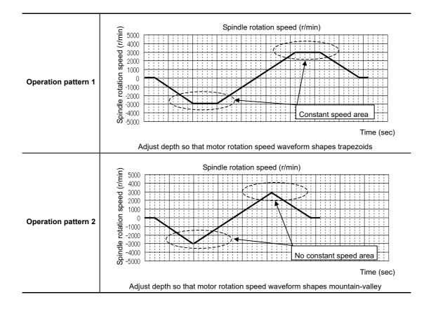
[3] Select "Synchronous tapping error measurement" on NC Analyzer, and perform synchronous tapping operations with the operation pattern 2 above.
