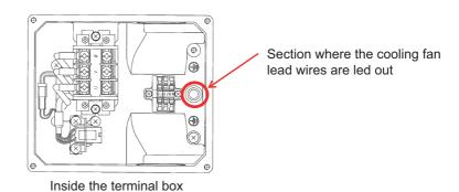
(b) Draw the lead wires including the protection tube of the cooling fan unit into the terminal box not to project at the back side of the motor. Failure to observe this could lead to breakage of the lead wires.
