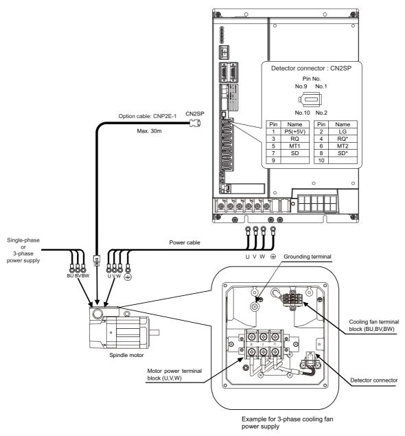
(Note) Either a single-phase or 3-phase power supply is used for the cooling fan. Refer to the Spindle Motor Specifications for details.
