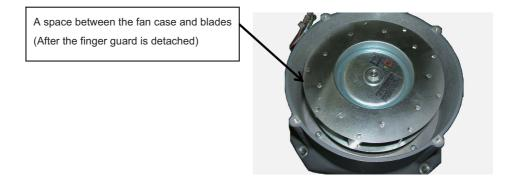
[5] Use the cleaning jigs to clean the air ducts of the spindle motor body.
