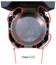
Motor frame's air ducts (cleaning points)
