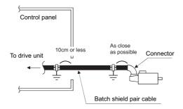
Encoder cable for servo motor
