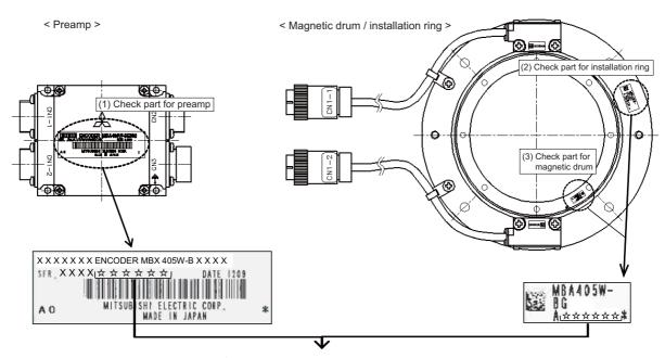
Make sure that the serial Nos. (☆ 6 digits) of the nameplate stickers attached on the above three parts are the same.
