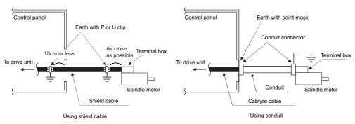
Power cable for spindle motor
