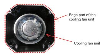
Cooling fan unit (after the bellmouth is removed)
