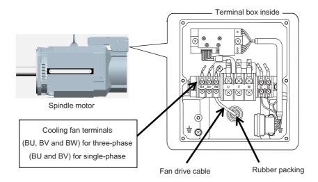
[2] Detach the cooling fan unit from the spindle motor.
