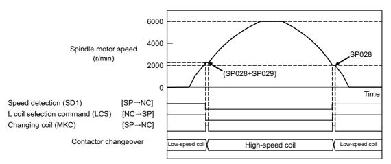
Spindle motor coil changeover control
