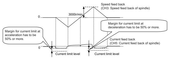
Output waveform example during synchronized tapping
