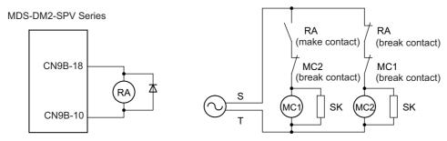
Coil changeover relay control circuit
