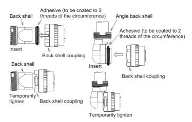
When tightening temporarily, match the concavity and convexity
