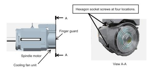
When slowly removing the cooling fan unit from the spindle motor, also unplug the fan drive cable slowly with the rubber packing left in the terminal box.
