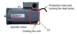
(Note 1) Do not strike the side face of the cooling fan unit. Failure to observe this may result in damages of the fan unit.
