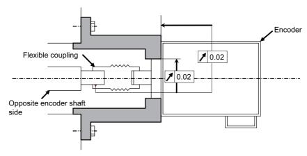
**Encoder and coupling installation accuracy**
