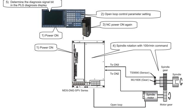
Installation diagnosis for spindle side PLG encoder
