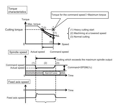
Allows the speed lowering and continues the machining
