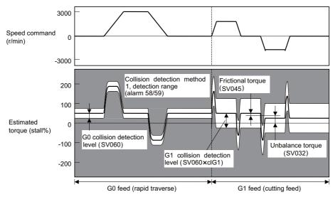
Alarm detection range for collision detection method 1
