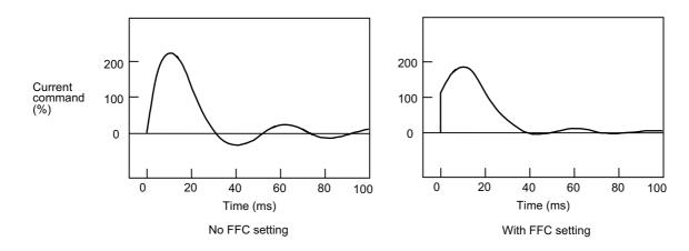
Acceleration rate feed forward gain means that the speed loop gain during acceleration/deceleration is raised equivalently. Thus, the torque (current command) required during acceleration/deceleration starts sooner. The synchronization precision will improve if the FFC of the delayed side axis is raised between axes for which high-precision synchronous control (such as synchronous tapping control and superimposition control).
