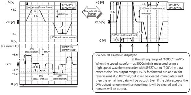
Example of D/A output waveform: 3000r/min during acceleration and deceleration
