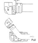
Work will become easy when the crimping part of the ground clip is pushed and the cable is bent as shown in the right figure.
