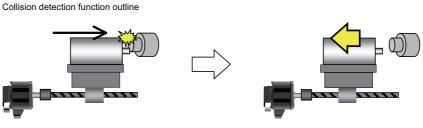
(a) A collision of machine is detected.
