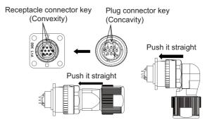
To remove, rotate the coupling and pull out to straight.
