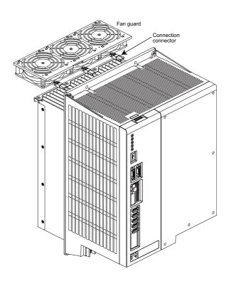
[3] Disconnect the fan connection connector.
