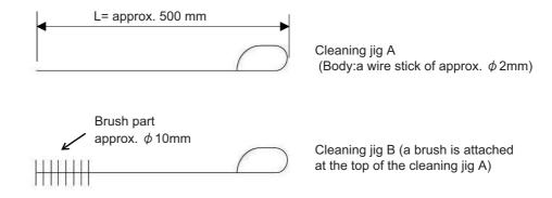
[3-2] Use the cleaning jigs to clean the air ducts of the spindle motor frame.
