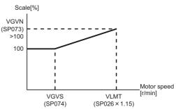
When lowering the speed loop gain at high speed
