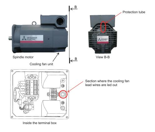
(Note 1) Take special care not to damage the lead wire for the cooling fan.
