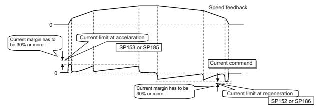
Output waveform example in spindle synchronous mode
