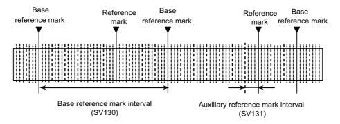
Incremental scale of distance-coded reference scale
