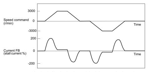
Acceleration/deceleration characteristics during conventional control
