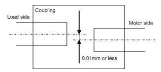
Also note that the motor side ball screw bearing must be locked so that to avoid the thrust load on the motor shaft due to expansion and contraction of the ball screw.
