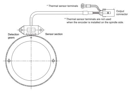
Spindle side PLG serial output encoder TS5690 Series
