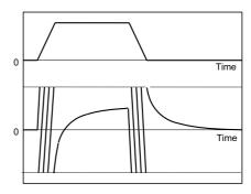
Vibration waveform with lead compensation control
