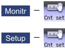
An arbitrary value can be set in the relative position counter which opens as a pop-up window. The counter cannot be set for an axis of auxiliary axis state. It also can be set on the setup (Setup) screen.
