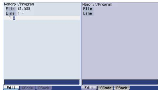
**Operation method (Creating a new machining program (When the parameter "#1285 ext21/bit2" is set OFF and the 1st part system is set as the displayed part system))**
