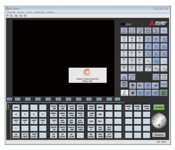
(Note) When the NC is running, the NC will be stopped. When the setting of [Tool (T)] - [Confirm NC Data Storage (N)] on the menu bar is enabled, the confirmation message to save NC data appears before NC is stopped.
