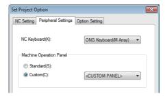
The setting of the custom machine operation panel of the imported project cannot be changed with NC
