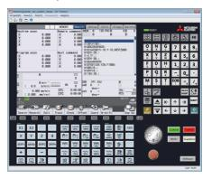
(Note) As the view mode (standard display mode / multi-window display mode) is retained, the screen is displayed in the mode previously selected.
