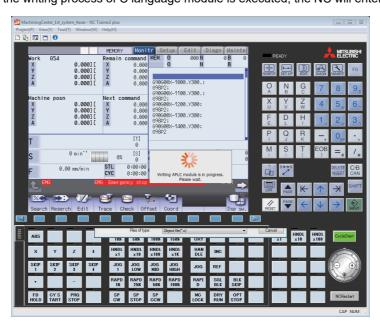
(5) The message box will appear after completing the writing process of C language module. To enable APLC, restart the NC with NC Restart button.
