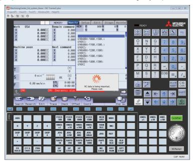
(6) When NC data import is completed, a message box is displayed. Press the [OK] button and restart the NC.
