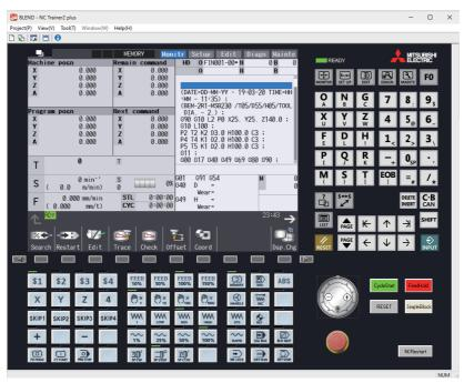
(2) Enable "[Tool (T)] - [NC Virtual Simulator Collaboration (V)]" in NC Trainer2 plus. The enabled/disabled status is saved as project data when changed.
