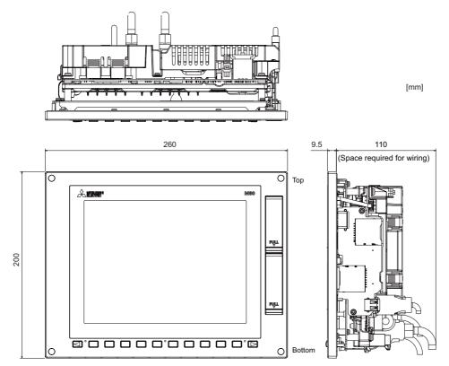
(Note 1) The 8.4-type display unit is incompatible with the touchscreen.(Note 2) The figure above shows the state with the graphic control unit mounted.
