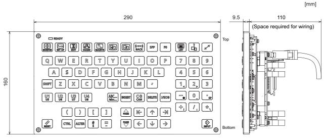
(Note) The above side view shows the state with the operation panel I/O unit mounted.
