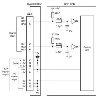
(Note) 12V power is separately required to connect 12V manual pulse generator. (Refer to "6.9 Connecting the Manual Pulse Generator".)
