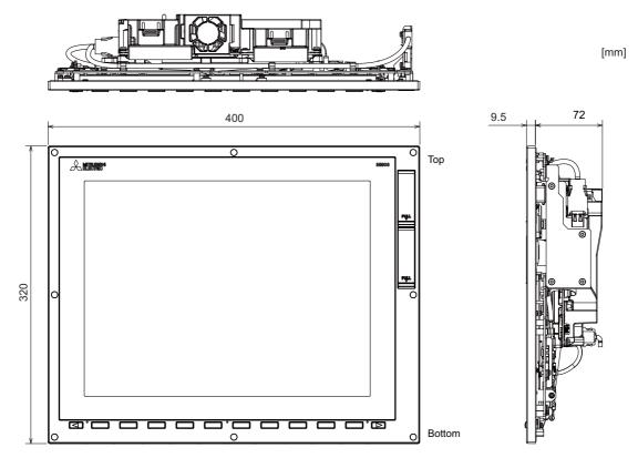
(Note) The figure above shows the state with the personal computer unit mounted.
