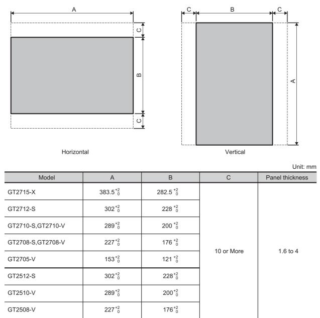
The C dimension shows the measurements for installing fittings on the control panel.
