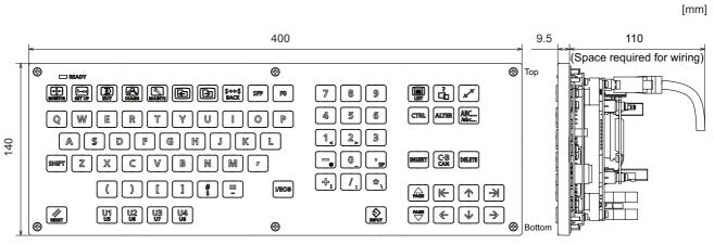
(Note) The above side view shows the state with the operation panel I/O unit mounted.
