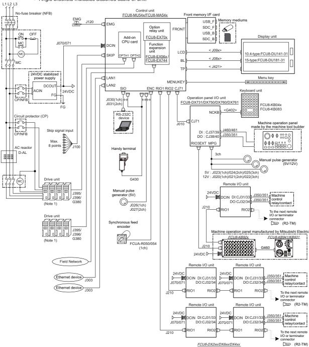
Dotted lines indicate the sections prepared by the machine tool builder.
