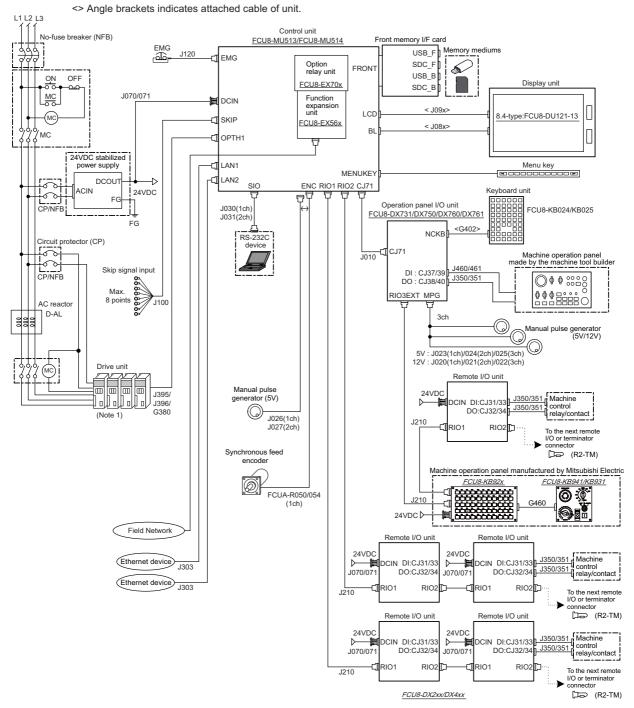
(Note 1) For information on how to connect the drive unit, refer to the drive unit's manual.
