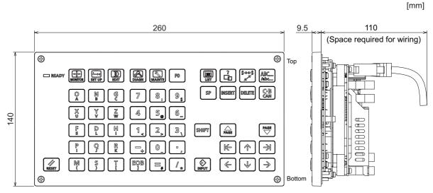
(Note) The above side view shows the state with the operation panel I/O unit mounted.
