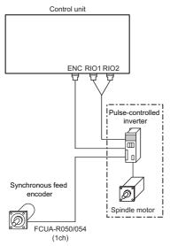
(Note) When the pulse-controlled inverter is connected, the remote I/O unit cannot be connected to the either of the RIO1 connector or the RIO2 connector.
