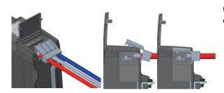
(3)Tilt the optional cover (EX-COVER-2) to fit it in the groove of the case.
