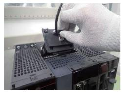
(3) Hold the connector on the end of the fan cable.
