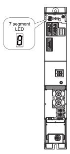
When the power of the NC and each drive unit/power supply unit is turned ON, each unit will automatically execute self diagnosis and initial settings for operation, etc. The LEDs on the front of the units will change as shown below according to the progression of these processes. If an alarm occurs, the alarm No. will appear on the LEDs. Refer to section "11.1.1 LED Display When Alarm or Warning Occurs" for details on the alarm displays.
