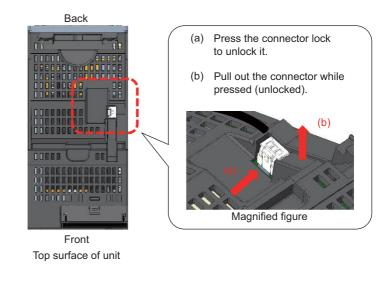
12.4 Replacing the Power Supply Unit Fan
