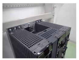
12.4 Replacing the Power Supply Unit Fan
