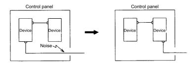
• Connect the control device earthing terminal and earthing plate with a thick wire. Take care to the leading of the wire.
