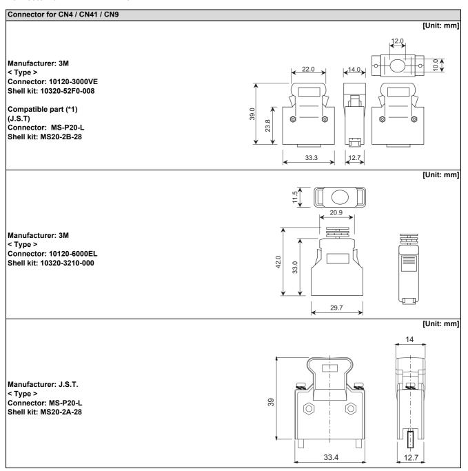
(\*1) The names of compatible parts may be changed at the manufacturer's discretion. Contact each manufacturer for more information.
