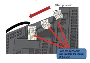
12.4 Replacing the Power Supply Unit Fan
