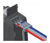
(2)Fasten the cables to the terminal block (L1, L2, L3) with screws.
