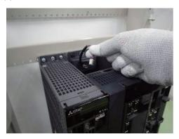
(4) Slide the fan connector down the slide and fix it.
