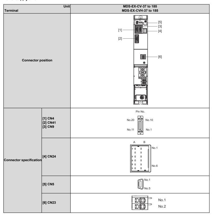
6.2 Main Circuit Terminal Block/Control Circuit Connector
