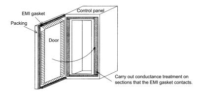
• As a method other than the above, the control panel unit and door can be connected with a plain braided wire. In this case, the panel and door should be contacted at as many points as possible.
