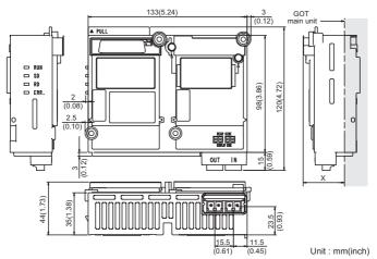
Dimensions of X when the CC-Link IE communication unit is mounted to the GOT.
