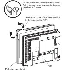
3) Starting from one corner, fit the other corners of the cover sequentially to the corners of the GOT, and then the sides (in the order of the arrows from A to D). Make sure that the gasket of the GOT rear face is entirely covered.
