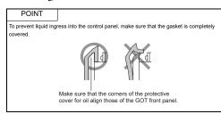
4) Mount the GOT onto the control panel. Mount the GOT once to control panels.
